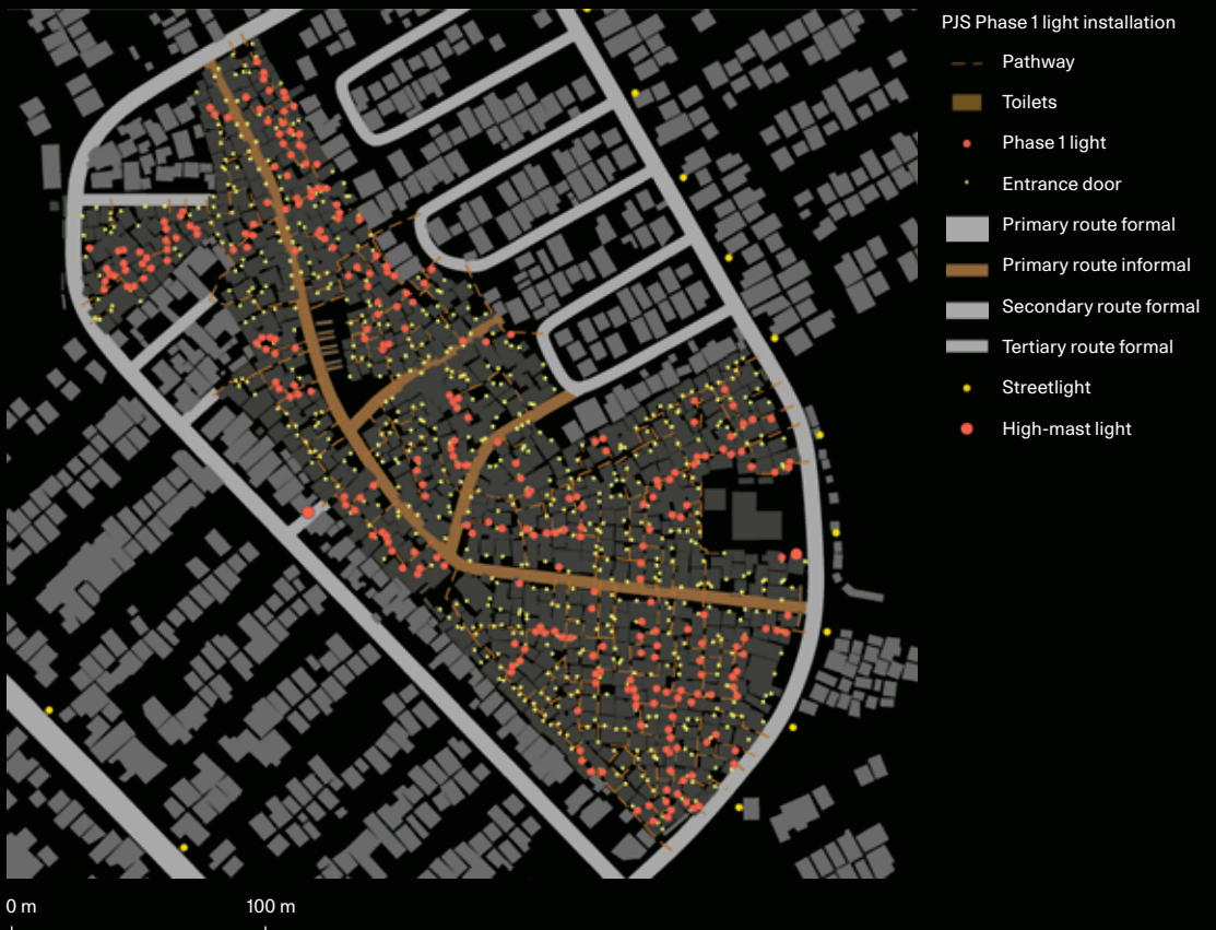
Map 1 Phase 1 lighting installation, with a light above or close to the front door of 283 households
