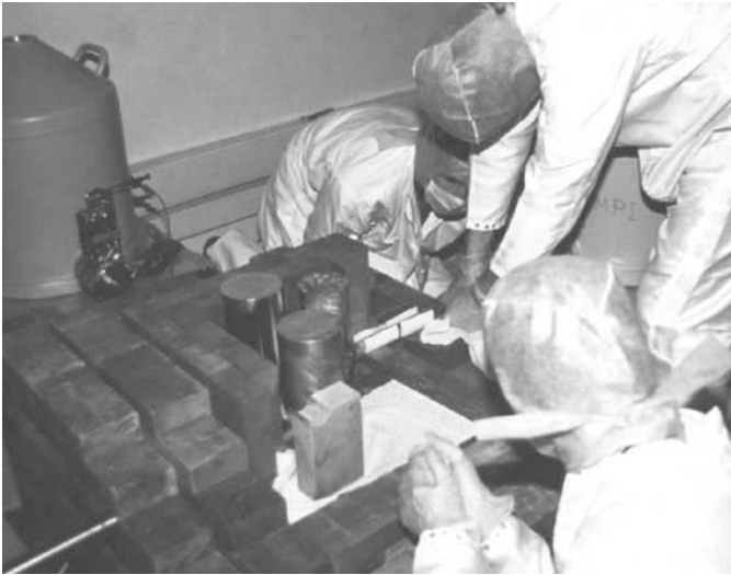
Figure 7.11. Photograph of a “classical” installation (detectors surrounded by shielding materials like copper and lead) of enriched detectors here exemplarily shown from the former Heidelberg-Moscow experiment. With kind permission of H. V. Klapdor-Kleingrothaus.
