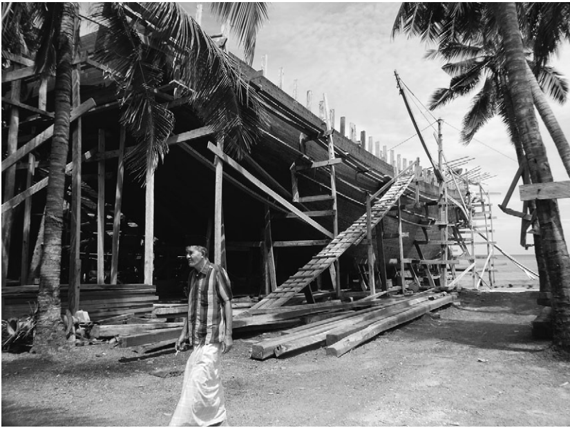
5.10 Bugis shipbuilding, Tanah Beru, Sulawesi, 2017. Photo: M. Fischer.
