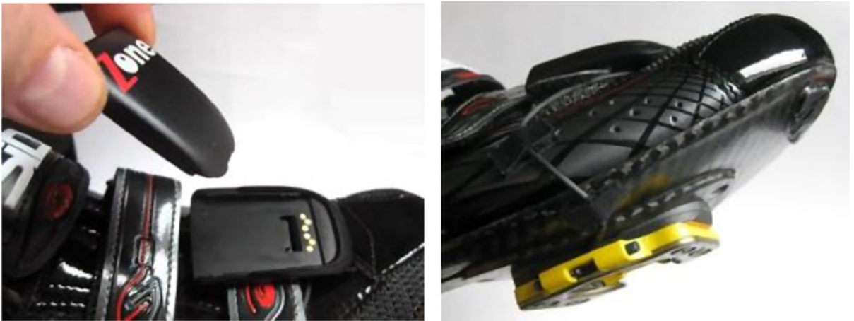
Figure 10-4. (a) Data collection pod, (b) strain gauge sensors attached to cleat (image used with permission from Brim Brothers)
