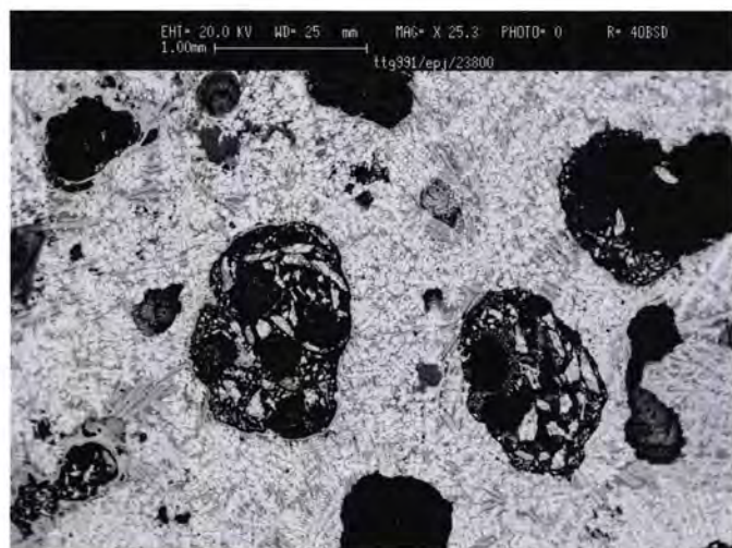
a SEM-BS image of TTG99.1 (RF 3956b) showing a three-phase polished block consisting of needles of fayalite, globular wustite and an interstitial phase, which is non-crystalline. Chemical analysis and the appropriate mineralogy suggest that this is a fragment of bloomery slag (bar = 1mm)
