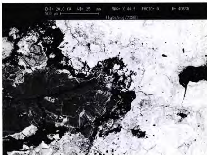
b SEM-BS image of TTG99.3 (the same sample as above), focusing on the area of the iron silicate inclusion (bar = 500 microns)
