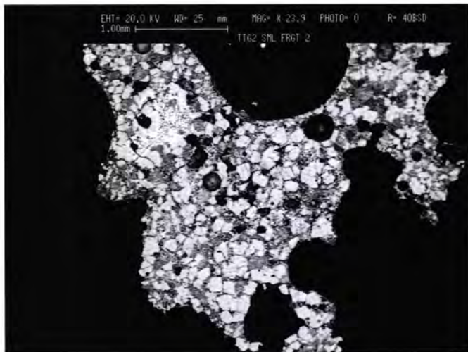
a SEM-BS image of sample TTG1/2 RFs 4337/4339, showing fragmented fayalite, hercynite and interstitial glass (bar = 1mm)
