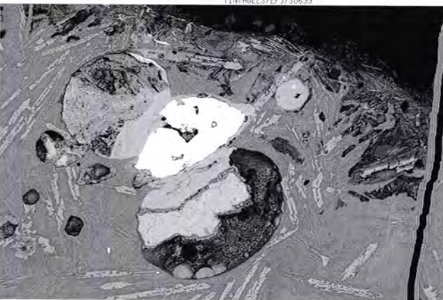
c SEM-BS image of a section of RF 1758 (TINT 3), the highly vitrified area. The bright metallic iron inclusion in the centre of the image and the ghost images of other round iron inclusions, presently weathered, suggests that this fragment was part of a furnace-wall (bar = 200 microns).
