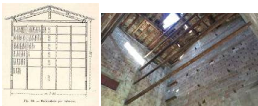
Fig. 2.1 Dryers kilns for tobacco: schematic cross-section of the building and interior layout of the uprights and crossbars for the “stendaggio” of tobacco; and current status of one of the studied dryers.
