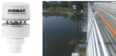
Fig. 2 Wind sensor 150WX, (AIRMAR, 2020) installed in test bed
