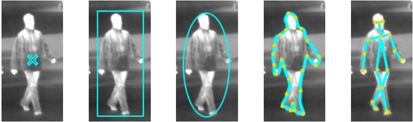
Figure 2.2: Examples of object states for different visual tracking tasks.
