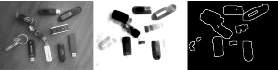
Figure 2-5. Another sequence of morphological pre-processing steps preceding polygon shape measurement: (Left) Original image. (Center) Range thresholded and dilated red color channel. (Right) Morphological perimeter shapes taken above a threshold
