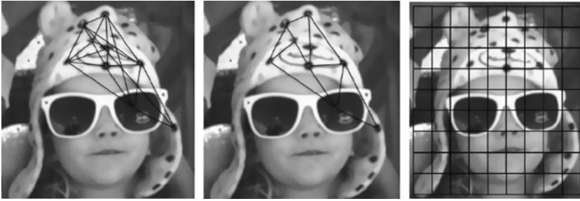
Figure 4-7. Reduced resolution examples of the D-NETS [135] sampling patterns. (Left) Full dense connectivity at interest points. (Center) Sparse connectivity at interest points. (Right) Dense connectivity over a regular sampling grid. The D-NETS authors note that a dense sampling grid with 10 pixel spacing is preferred over sampling at interest points
