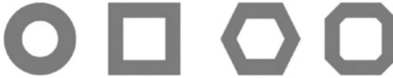
Figure 6-19. CenSurE bilevel center surround filter shape approximations to the Laplacian using binary kernel values of 1 and -1, which can be efficiently implemented using signed addition rather than multiplication. Note that the circular shape is the desired shape, but the other shapes are easier to compute using integral images, especially the rectangular method
