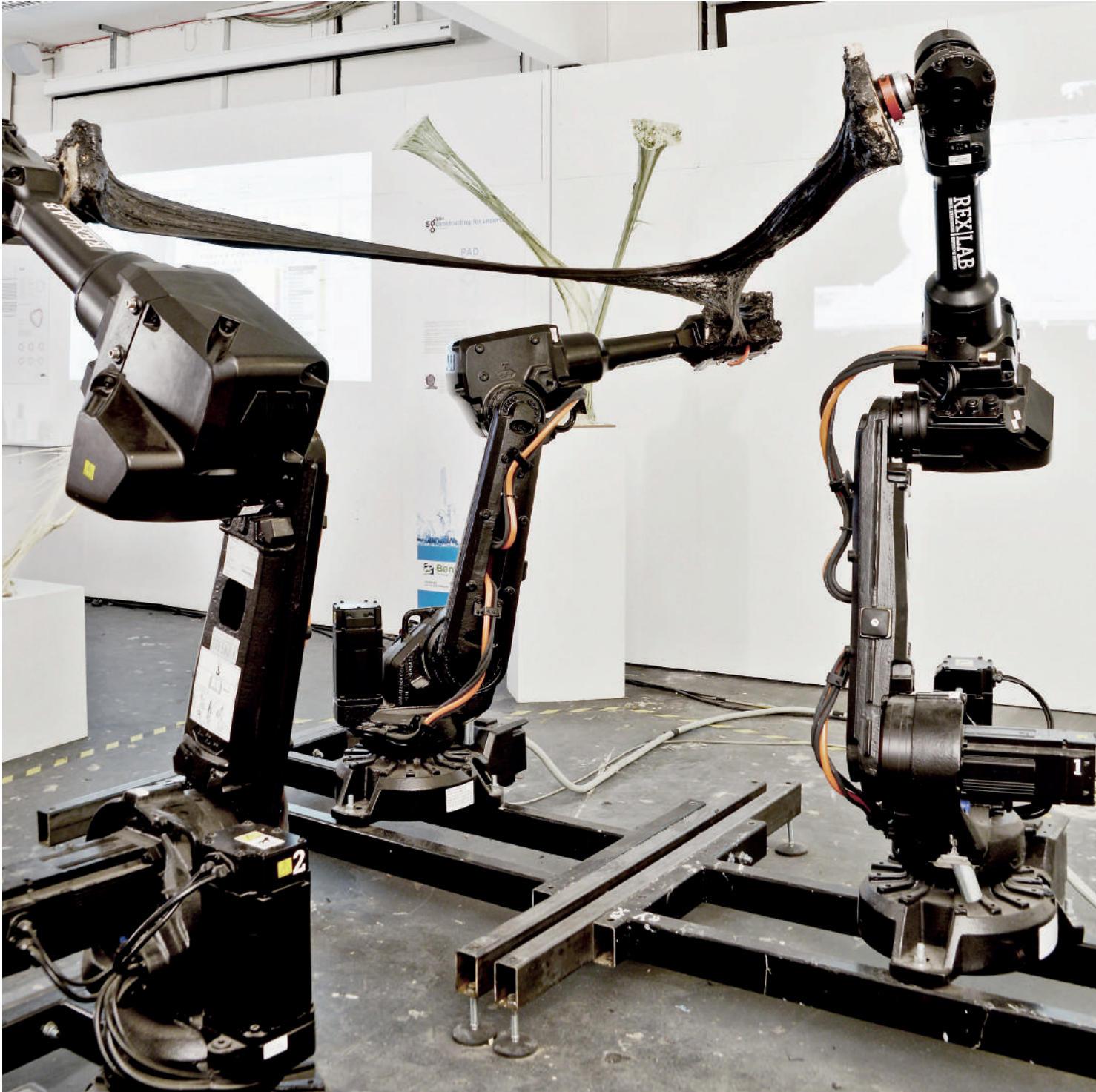
Fig. 1: REX|LAB at the Bartlett School of Architecture, demonstrating the material process of stretching soft foam into self-supporting filamentous structures. Event: Robotic FOAMing, Smartgeometry 2013.
