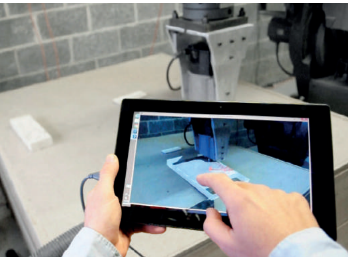
Fig. 4: Interactive milling: The robot's toolpaths are overlaid with live video of the milling operation. Touching an area of the screen causes the robot to immediately move to and mill in that area.
