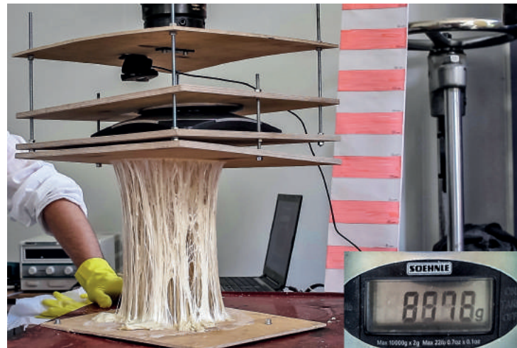
Fig. 12: Feedback on internal forces to predict material failure. Event: Responsive Robotic Materialization Workshop, Estonia 2013. (Photo: Markus Brandtner.)
