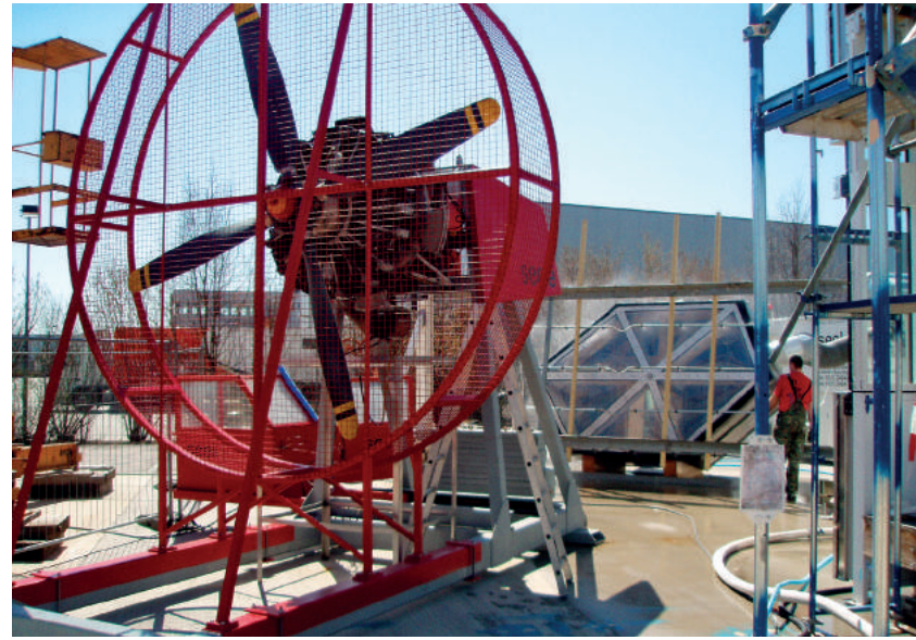
Fig. 8: Performance test of node connection with six ETFE cushions with low negative pressure in the chamber and full wind deflection with an aircraft propeller simulated storm. (Photo: se-austria.)
