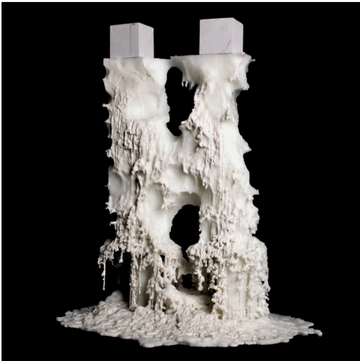
Fig. 10: Wax model. Two downward loads and asymmetric supports.
