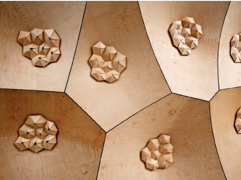
Fig. 3: Photos of the hygroscopic apertures in different states. a) High relative humidity, 75%. b) Low relative humidity, 45%.
