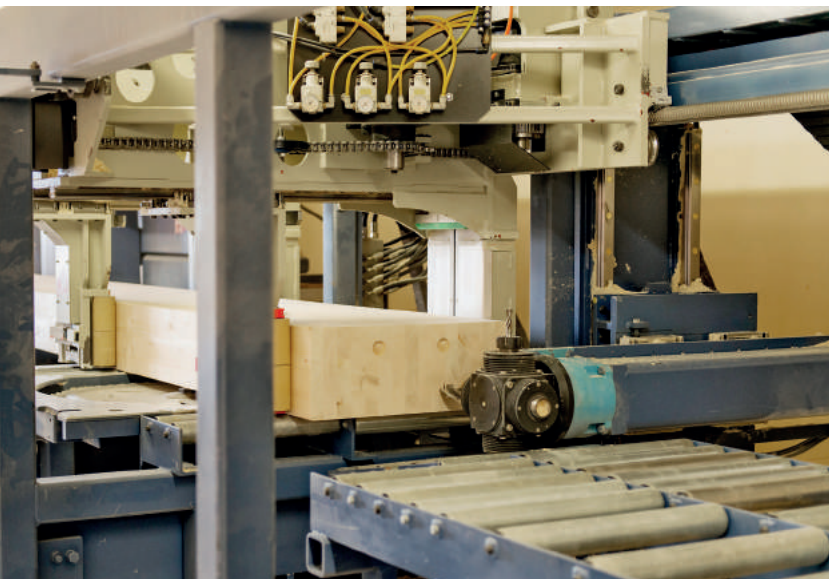
Fig. 7: Photograph showing five-axis computer numerical control (CNC) robot slotting machine used to cut the beams to length and machine all required workmanship, including blind holes and milling grooves. Wiehag Factory, Altheim, Austria. (Photo: Mitterbauer.)
