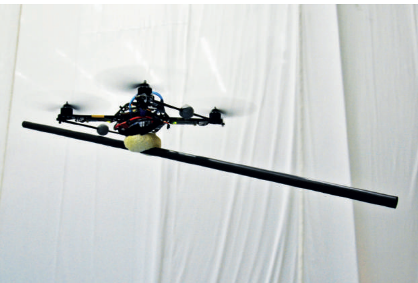
Fig. 3: a) Lightweight jamming gripper for the assembly of space frame structures. b) Cable dispenser tool for the erection of tensile structures.
