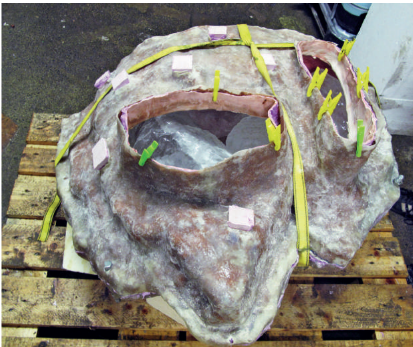
Fig. 12: A completed mould, resealed, shelled and loaded with stock ice. The mould is then filled with water and fitted with pumps to ensure a slow, clear freezing process.
