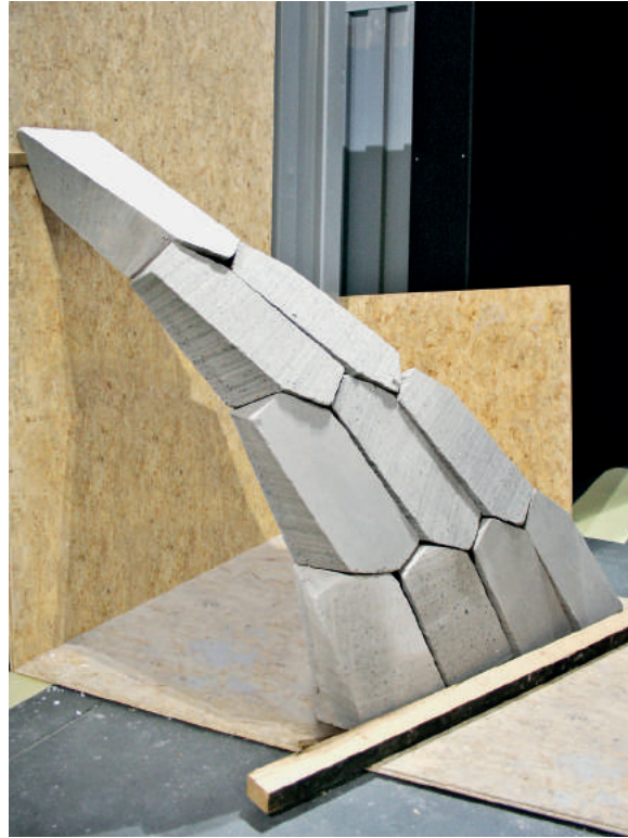
Fig. 3: Initial test cuts in engineered limestone.
