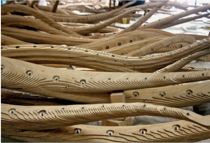
Fig. 7: Rows of assembled branch slices awaiting tensioning into trunk slots.
