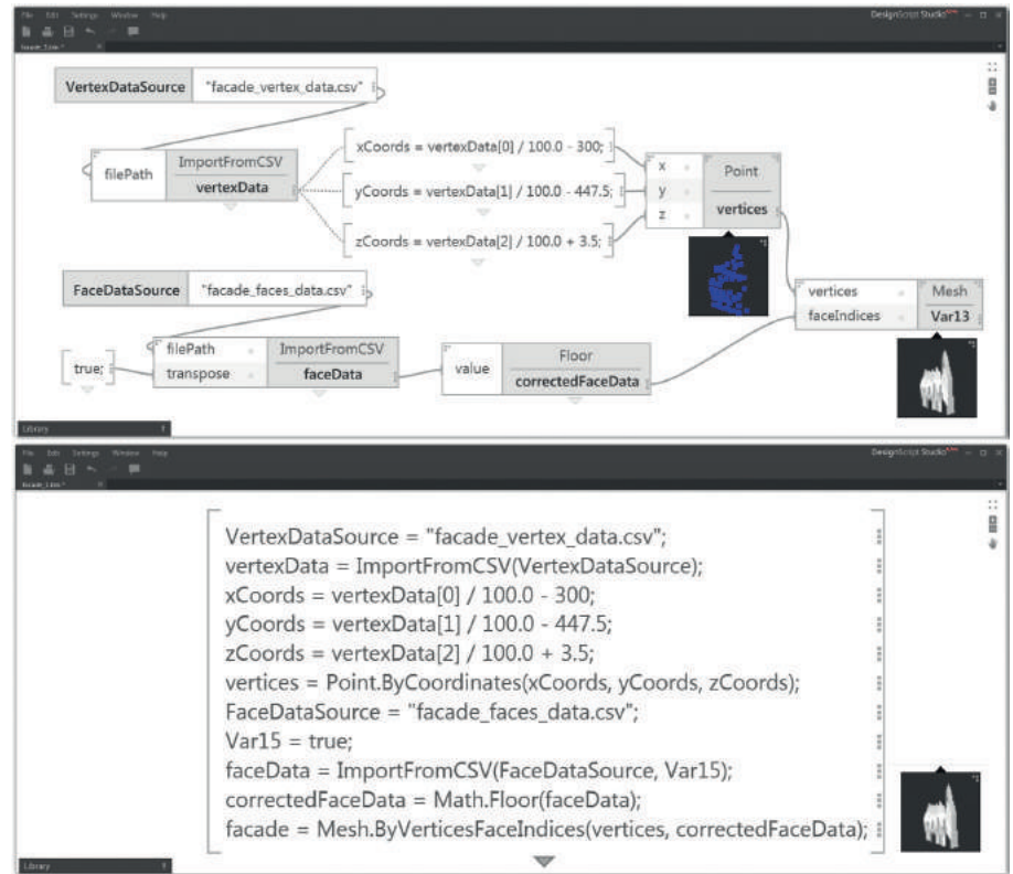
Fig. 14: Diagram outlining DesignScript data flow graph used as a visual programming interface (top) as well as its 'node to code' functionality (bottom), allowing the designer to selectively replace all or part of a graph node diagram with the corresponding code, thus making it possible to reduce visual clutter and progress to a more succinct form of design computation.
