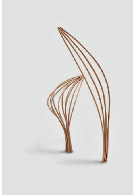
Fig. 8: The formed curve is not affected by the gravity force. No support material is needed. (Image by courtesy of Joris Laarman Lab.)
