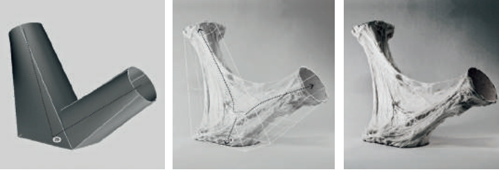
Fig. 4: Geometrically precisely defined design strategy translated into fully controlled robotic movements and reacting with loosely controlled material mixture results in unpredictable morphogenetic behaviour. Event: Robotic Infiltrations, Architecture Challenge 2013. (Image: REX|LAB.)
