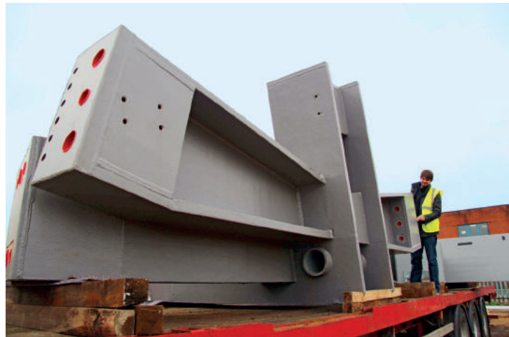
Fig. 9: Node 6 after the application of finishes, ready for component sign-off.
