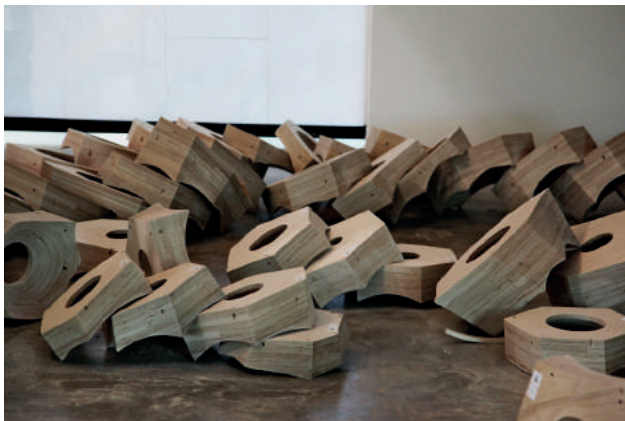
Fig. 10: Various unique voussoirs that compose the vault.
