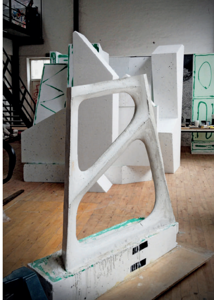
Fig. 10: Opticut 1:1 sample cast, testing the casting quality of two adjacent, doubly ruled cells.
