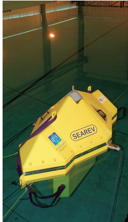
■ Photo 7 : autonomous electricity system for wave energy recovery (Searev) mock-up (© École centrale de Nantes, FR).
