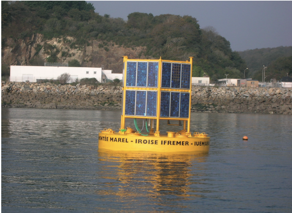
■ Photo 36 : Marel station for multi-parameter measurements; arrays of this type of buoy provide better information about the coastal environment and make it easier to monitor the impacts of any development (© Ifremer/TSI).
