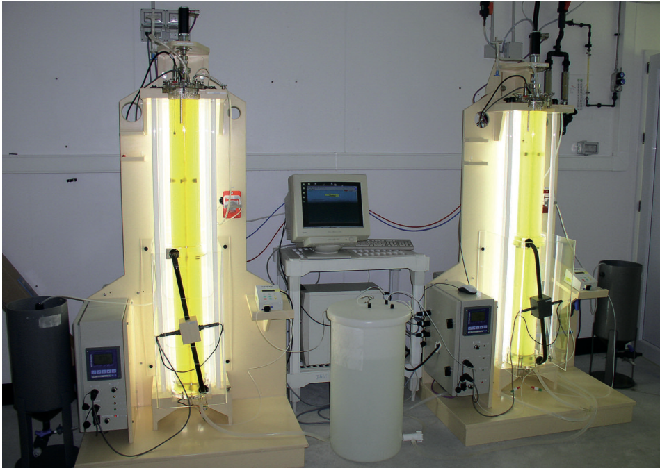
■ Photo 34 : photobioreactors holding 17 litres used to feed the bivalve mollusc larvae and juveniles (© Ifremer, J.P. Cadoret).
