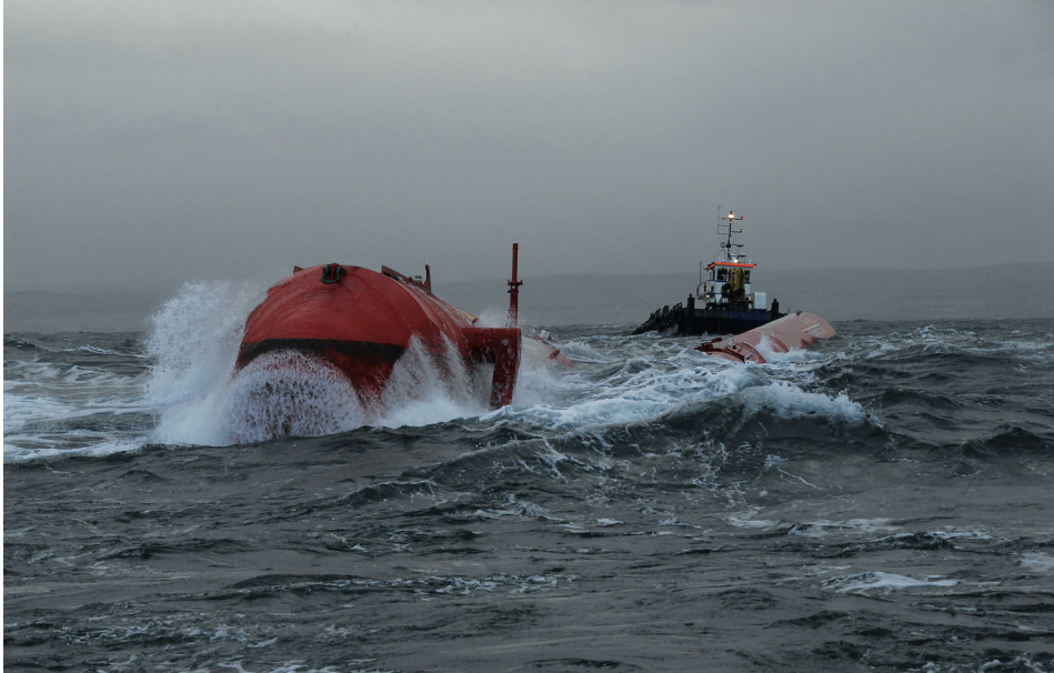
■ Photo 1 : the Pelamis system to recover wave energy being tested under rough conditions at the European Marine Energy Centre in Scotland (© Pelamis Wave Power Ltd, UK).
