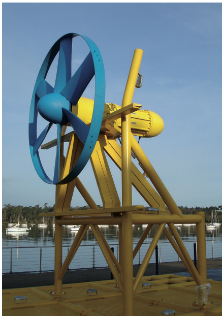
■ Photo 13 : Sabella stream turbine ready to be submerged in Brittany (© J. Ruer).
