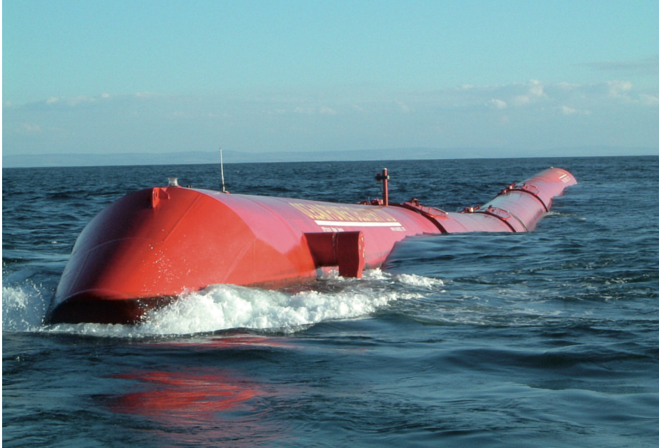
■ Photo 32 : Pelamis system to recover wave energy being tested under smooth conditions at the European Marine Energy Centre in Scotland (© Pelamis Wave Power Ltd, UK).
