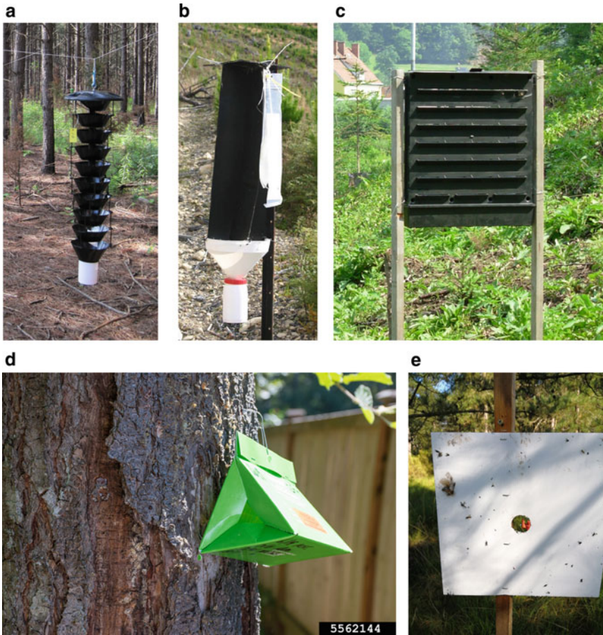
Fig. 19.6 Various traps used for insect monitoring and surveillance: a Lindgren-funnel trap. Credit: D. Miller, USDA Forest Service; b Panel trap with alpha-pinene and ethanol lures attached. Credit: J. Kerr, Scion, New Zealand; c Theysohn bark beetle trap. Credit: Gernot Hoch, BFW Institut für Waldschutz, Vienna, Austria; d Delta trap. Credit: Karla Salp, Washington State Department of Agriculture, Bugwood.org ; e Sticky plate trap with pheromone lures in the center and a trapped pine processionary moth. Credit: Hervé Jactel, INRAe, France
