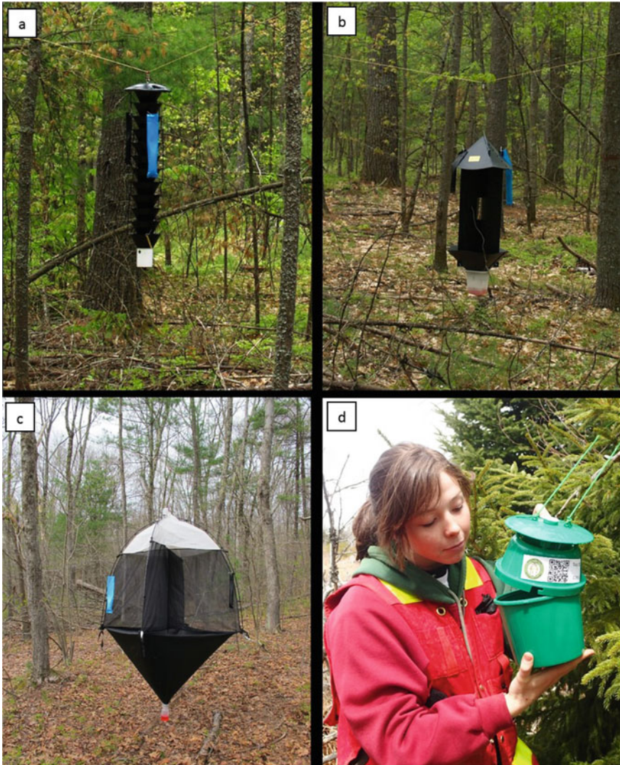
Fig. 17.3 Examples of traps used to survey for forest insects: a multiple funnel and b intercept panel traps are commonly employed to survey for bark beetles and woodborers; c canopy malaise traps are used for bark beetles and woodborers as well as other taxa (Photo credits: K. J. Dodds); and d Unitraps are used to collect Lepidoptera (Photo credit: M. MacDonnell, University of New Brunswick, Fredericton, NB)
