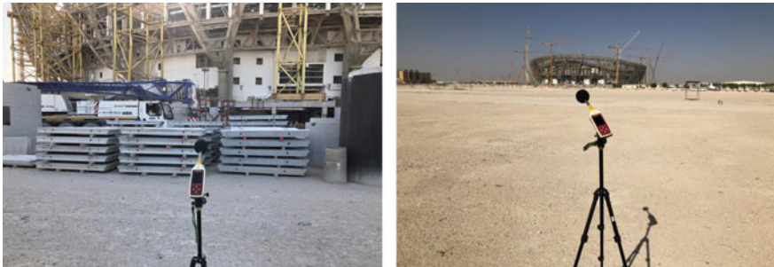
Fig. 7.5 Noise testing around the stadium
