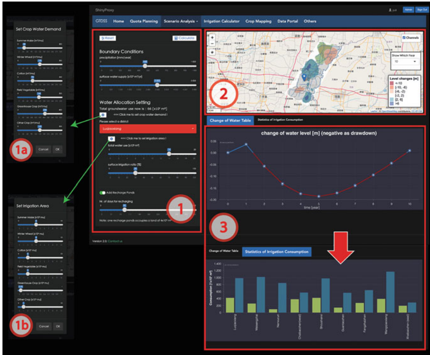
Fig. 4.47 Interface of the 2-D groundwater modelling tool. Panel 1 provides comprehensive input options to specify boundary conditions and the allocation settings on a township basis. For each township, users can also define landuse and crop water demand via panels 1a and 1b, respectively. Panel 2 is the output window for the spatial map of simulated groundwater level change. Panel 3 displays the time-series of level change at a selected location, as well as the water allocation results per township
