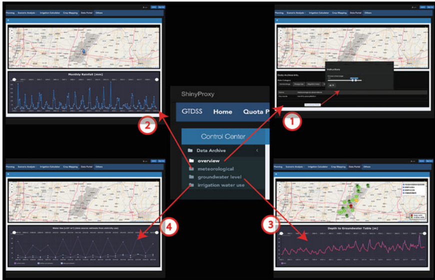
Fig. 4.50 Interface of the data portal module. Panel 1 shows the data inventory and options for downloading data items individually. Panel 2 shows the plot of monthly precipitation time-series. Panel 3 allows users to visualize time-series of depth to groundwater table at different monitoring wells shown on the map. Panel 4 plots water use time-series estimated from electricity consumption.
