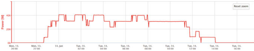
Fig. 4.21 Time series of the working power showing status of pumps connected to one transformer (In this example 4 pumps are connected to the transformer)
