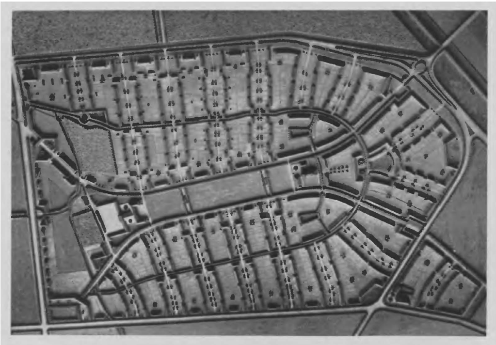
FIGURE 1.8.1 Plan of the Zimpel settlement in Breslau commissioned by the Siedlungsgesellschaft Breslau A.G. to architects Paul Heim and Hermann Wahlich in 1919: The south-west-northeast middle axis comprised a number of communal buildings aligned along a central garden.
