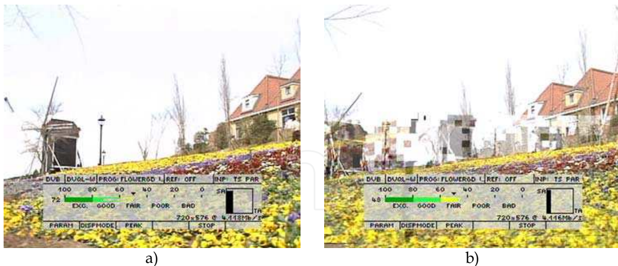
Fig. 9. Example of a real-time objective picture quality analysis using DVQ analyzer. The metric DVQL-W is used to demonstrate the achieved video image quality in one frame of the a) reference video, b) degraded video with blockiness and cliff-off effect present.
