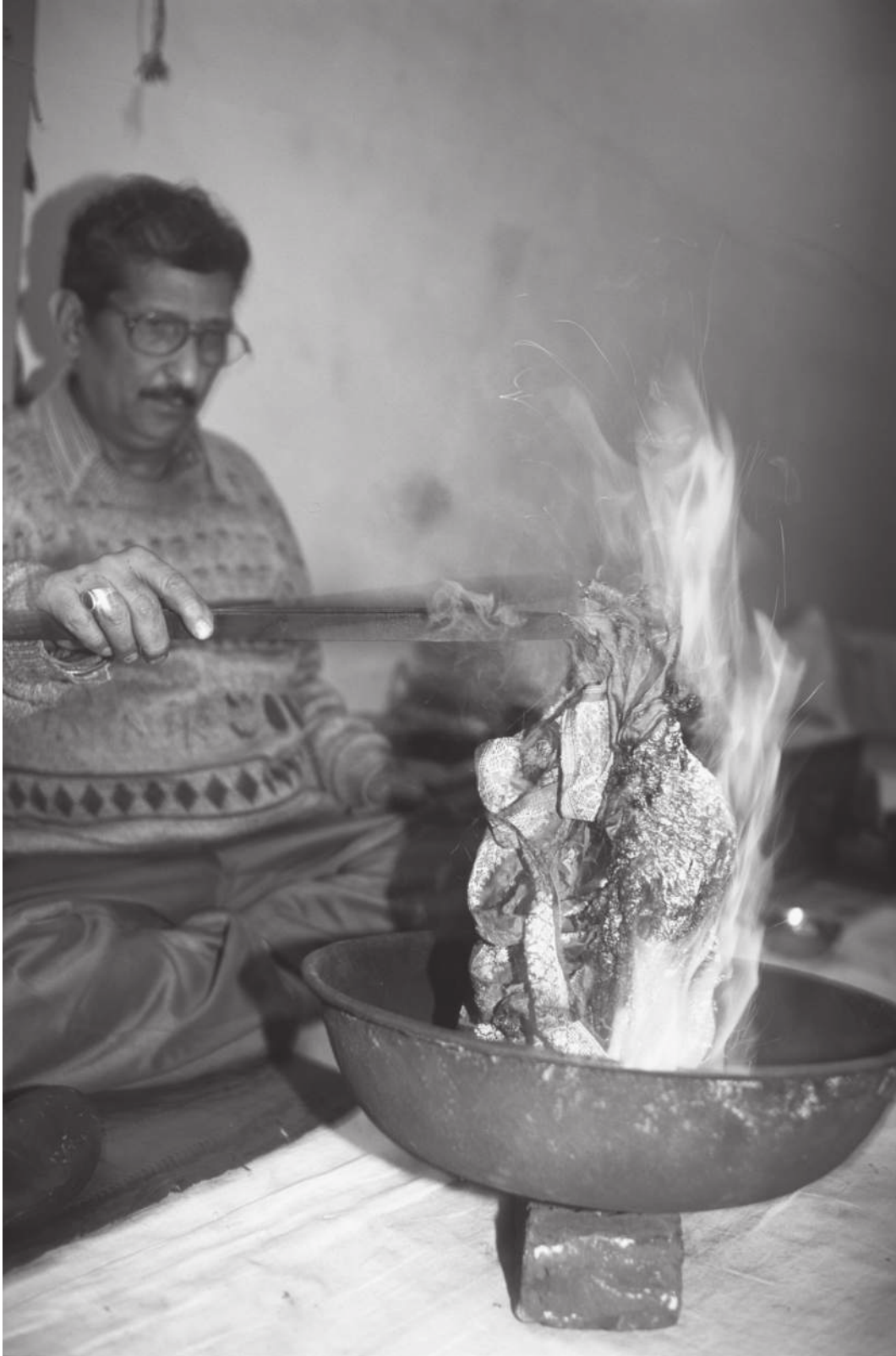
Figure 12.4. Dealers in Old Delhi's jewellery market test the metal threads used to decorate silk saris for purity, then burn the clothing to reclaim the silver and gold (© Tim Mitchell and Lucy Norris).
