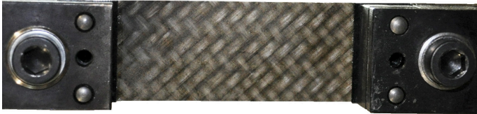
Figure 5.18: Tension test. Clamping device with 36 mm specimen, undeformed configuration.
