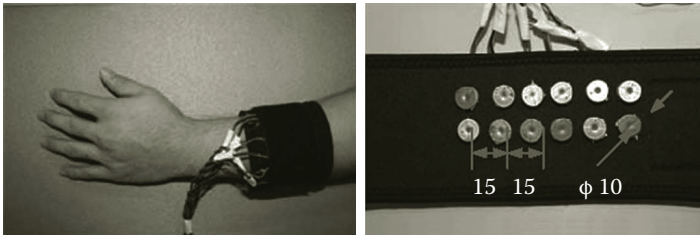
FIGURE 12.2 Multichannel sEMG sensor ring: (a) sensor ring on the forearm and (b) six-channel sEMG electrodes.
