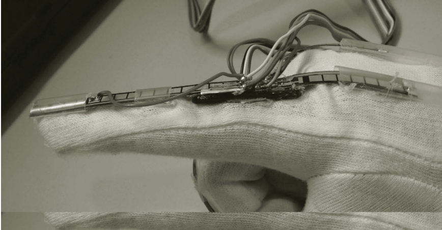
FIGURE 15.12 Data glove used for measurement of DIP and PIP joint angles.
