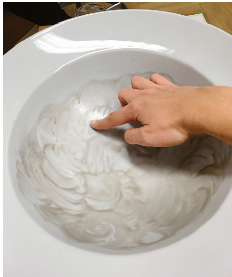
Fig. 2: Grinding silver leaves by hand together with gum arabic in a porcelain bowl, until the silver is finely dispersed.
