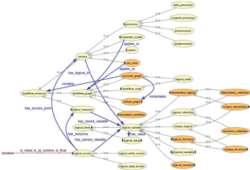
Fig. 3.3 Workflow resource branch fragment of the OSMO class hierarchy, version 1.6.8. The OWLviz protégé plugin was used to visualize the ontology [10]; arrows labelled “is-a” denote subsumption ( \sqsubseteq ), and the other arrows denote relations; solid line: datatype properties (flags) associated with the osmo:logical_access concept
