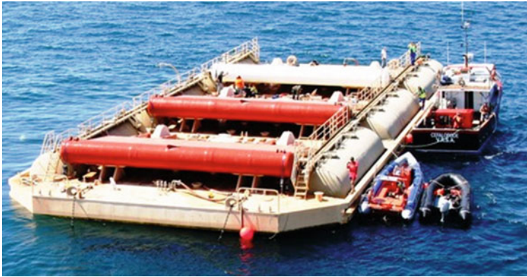
Fig. 2.18 Waveroller WEC prototype, before submerged to seabed [35]
