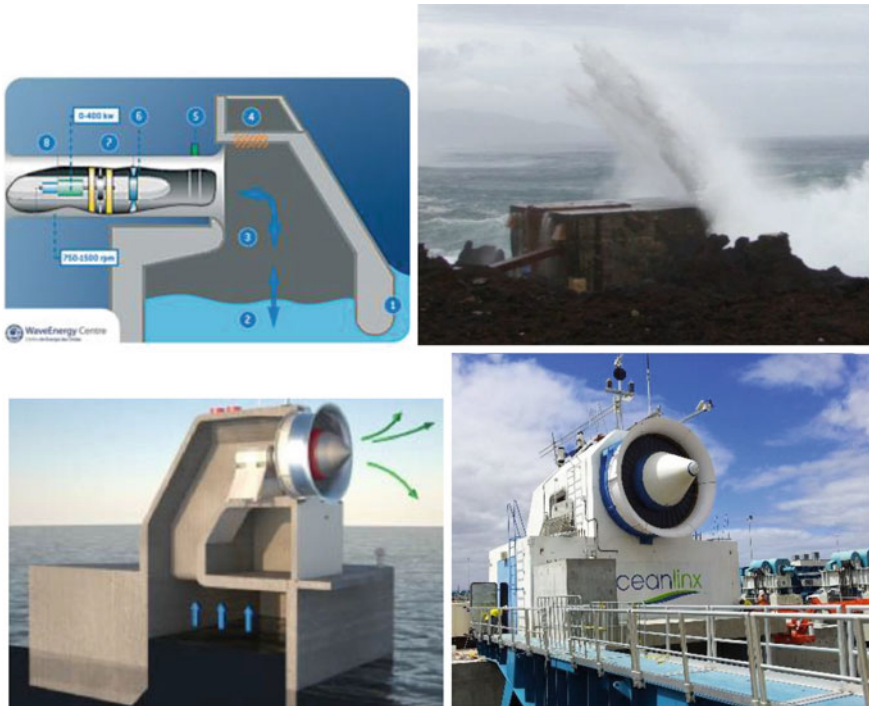
Fig. 2.7 The Pico OWC, schematics ( top, left ) and in action ( top, right ) [25], OceanLynx, schematics ( lower, left ), and in real life ( lower, right ) [26]
