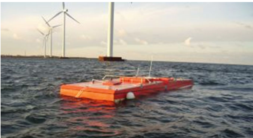
Fig. 2.10 Crestwing , at a scale of 1:5, tested near Frederikshavn during autumn 2011 [28]
