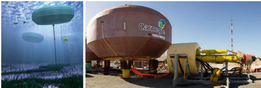
Fig. 2.16 Carnegies CETO . A submerged tether moored point absorber [33]
