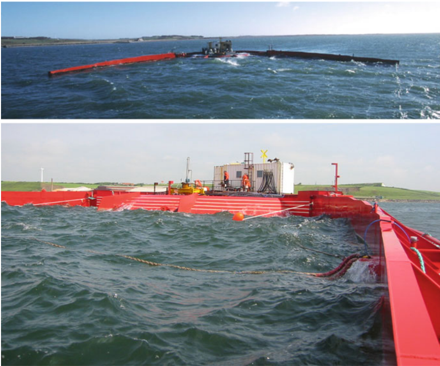
Fig. 2.24 Wave Dragon 1:4.5 scale grid connected prototype tested in Nissum Bredning, Denmark
