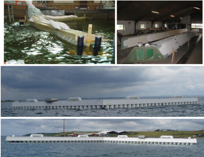
Fig. 2.8 Leancon 1:40 scale model in wave basin ( top, left ), 1:10 prototype for testing in Nissum Bredning, Denmark, under construction ( top, right ) and after deployment ( middle and bottom ). Courtesy of LeanCon
