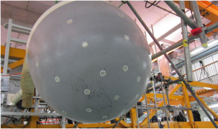
Fig. 9.18 Picture of a floater of the Wavestar WEC being experimentally tested for wave loads. Courtesy of Wavestar
