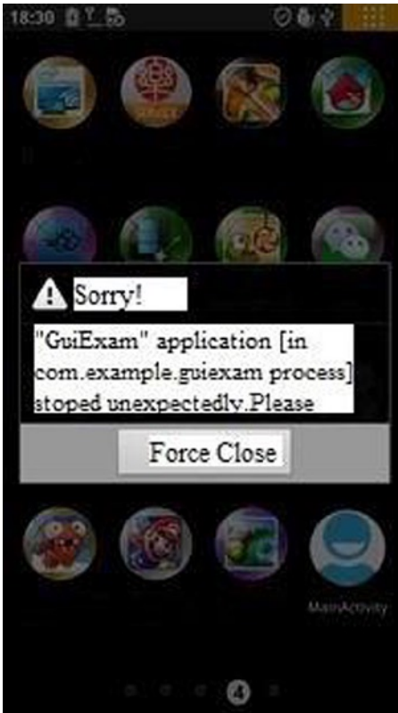
Figure 11-15. Running error when a worker thread directly calls a function of the UI object
