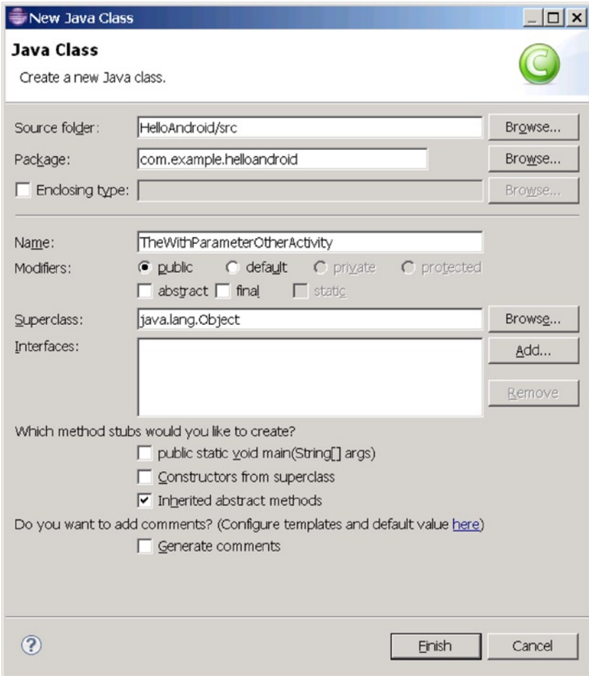
Figure 9-13. Add the corresponding class for the newly added layout file in the HelloAndroid project
