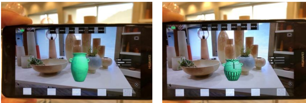
Figure 3: Simulating Dimensions, Colours, and Patterns (green virtual model incorporated in a real showroom; changing dimensions on the leftmost image and simulating patterns on the right)
