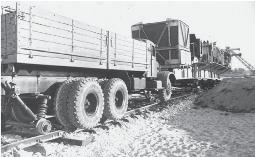
A KRAZ 218 lorry adapted for railway operation, with an SRK 20 crane, during the VISTULA 75 exercise, photo by Colonel J. Jarzyna (courtesy of Colonel J. Jarzyna)
