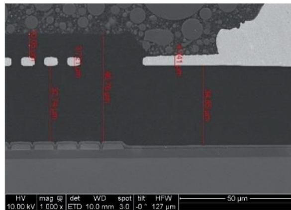
**Figure 4.** Cross section for the fabricated isolation transformer.
