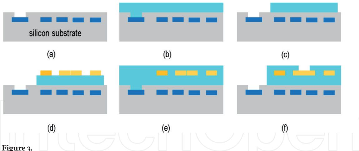
**Figure 3.** Isolation transformer process flow. (a) CMOS substrate with top metal, (b) polyimide layer spin coated, (c) polyimide layer patterned & cured, (d) top coil plated, (e) 2<sup>nd</sup> polyimide layer spin coated and (f) 2<sup>nd</sup> polyimide layer patterned & cured.
