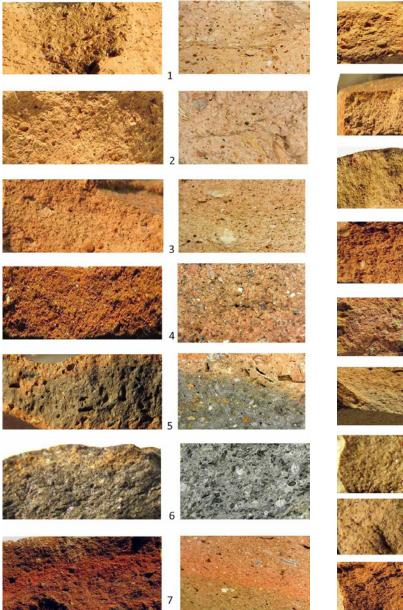
Figure 9.4. Fresh fractures of samples 1-7, left macro, right digital microscope, 100x.<sup>5</sup>
