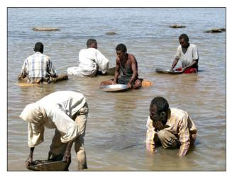
Plate 3.6. Nile, Abu Dis. Miners separate the gold flakes from the raw mineral.
