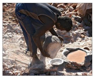
Plate 3.3. Jebel en-Nigeim, separation of gold from quartz powder.
