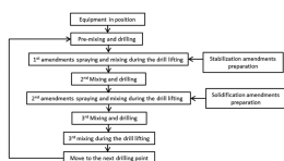
Figure 2. Engineering flow diagram of stabilization/solidification.
