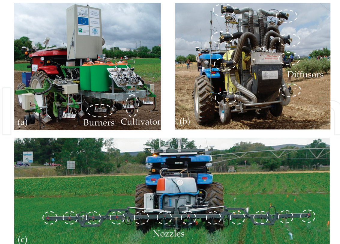
Figure 6. Implements working: (a) thermal and row cultivator, (b) canopy sprayer and (c) patch sprayer.
