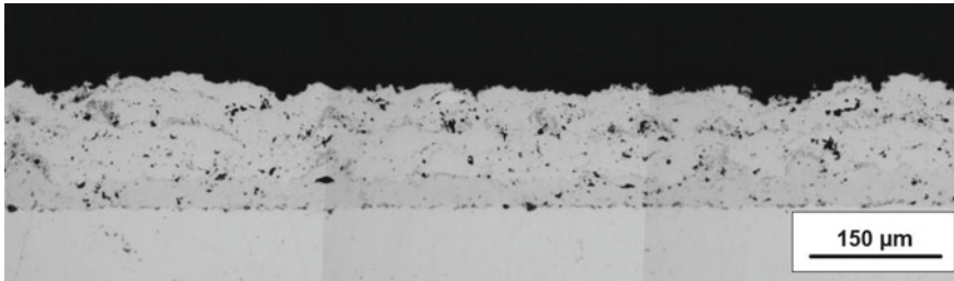
Fig. 4 Cross section of the coating after one cycle in the wind-tunnel experiment at surface temperatures of 1300–1350 K
