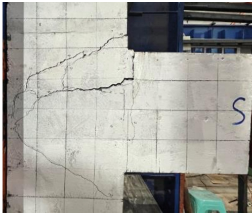
Fig. 18. SKL2 specimen tensile test failure diagram
