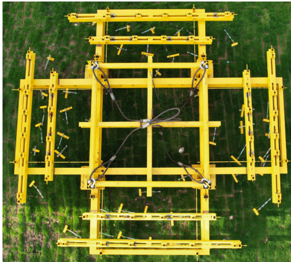
Fig. 4. Schematic diagram of the overall lifting spreader structure of the reinforced bar product.
