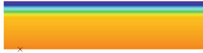
Fig. 29. Temperature distribution of the most unfavorable inner surface of the thermal bridge beam X_{Timn} = 16.6\text{ }^{\circ}\text{C}
