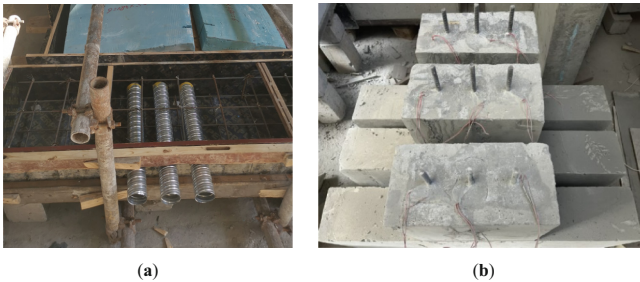
Fig. 7. Tensile test specimens with horizontal joint manufacturing progress: (a) Reinforcement fabricating; (b) Assembled and grouted specimens.
