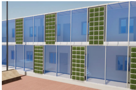
Fig. 3. Design illustration of prefabricated construction and vertical greening based on BIM technology
