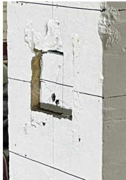
Fig. 13. LGS members slippage movement of SKJ2
