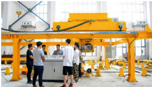
Fig. 1. Site for the production of PC components in prefabricated buildings
