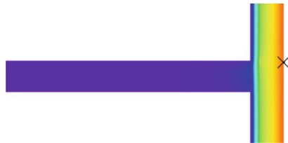
Fig. 31. Temperature distribution of the most unfavorable inner surface of the thermal bridge joint of the external floor slab X_{Timn} = 16.8\text{ }^{\circ}\text{C}
