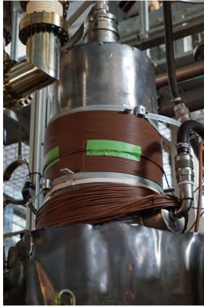
Figure 7.8: Additional collector coil for solving the limitation of the high body current.
