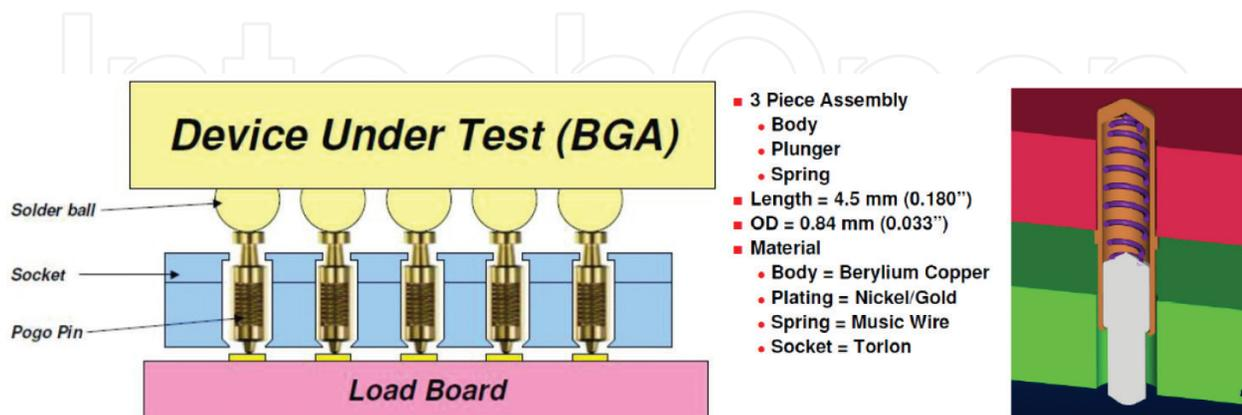
**Figure 16.** A pogo pin socket system overview.
