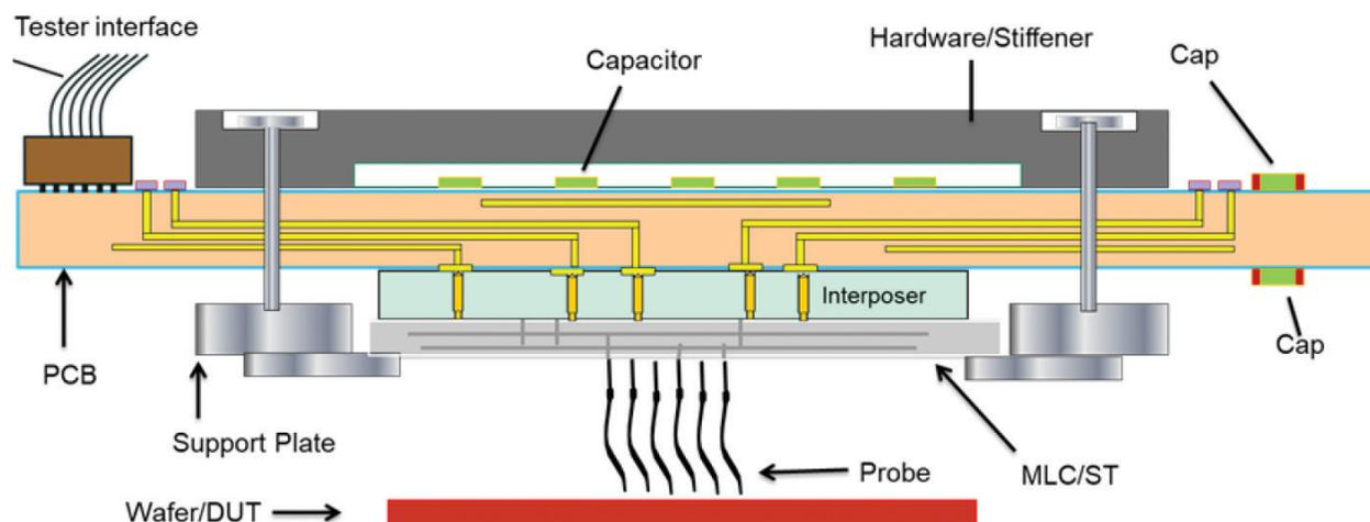
**Figure 1.** Probe card system architecture is shown.
