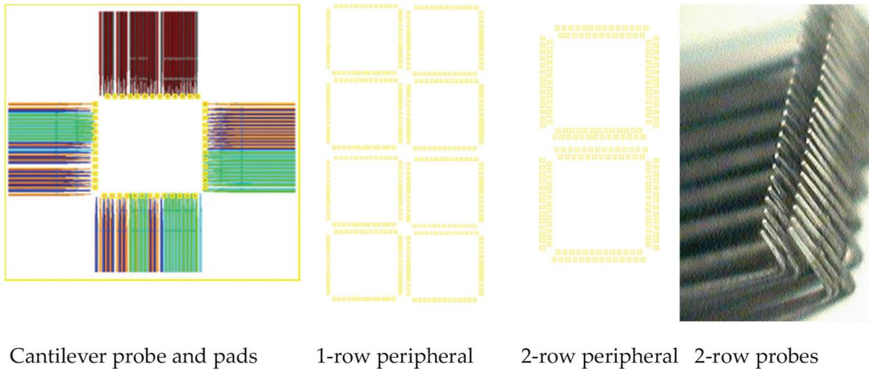
**Figure 3.** Cantilever design and contact pad layouts.
