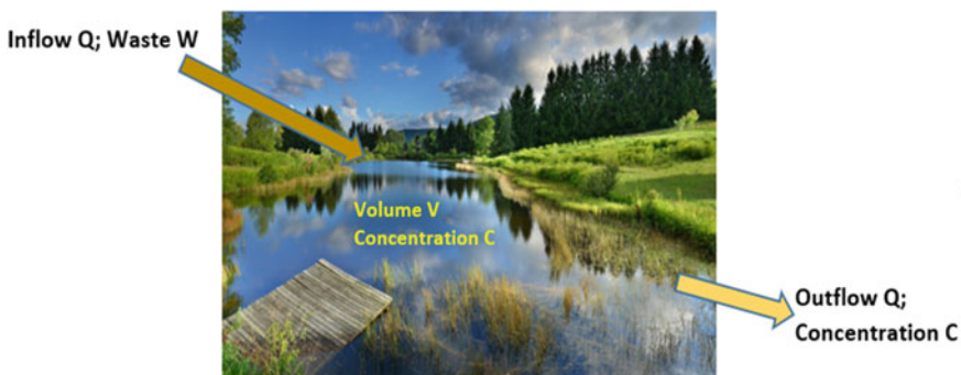
Fig. 15.2 A constant volume lake receiving wastewater containing a pollutant
