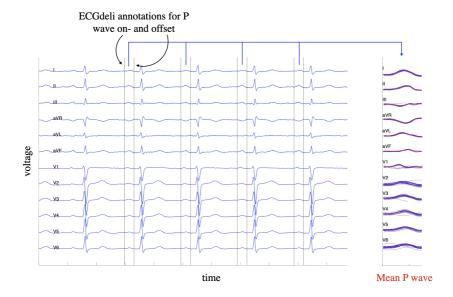
Figure 9.5: Averaging single beat P waves for each 12-lead ECG in the clinical dataset. This procedure was performed to obtain a mean P wave per subject and patient. An exemplary clinical 12-lead ECG is visualized in blue along with the ECGdeli annotations for P wave on- and offset in each beat. Averaging over all P waves detected in the signal trace resulted in a mean P wave template for each subject.
