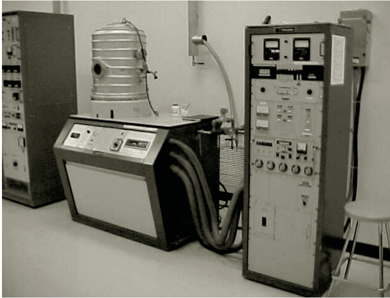
FIGURE 7.4 Thermal evaporation system. (Courtesy Edwards.)
