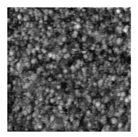
Figure 6.5. Constant-current STM images of Au(111)-films after 30' of immersion in a freshly prepared THF/NH<sub>3</sub>(aq) solution of 3 (setpoint=5 pA, bias=1.3 V).
