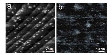
Figure 8.5. (a) STM image  $(100 \times 100 \text{ nm}^2)$  of DPPH molecules deposited on Au(111). Tunnelling current I<sub>t</sub>= 10 pA, Bias Voltage BV= 0.1 V. (b) STM image  $(15 \times 15 \text{ nm}^2)$  of BDPA molecules deposited on Au(111). I<sub>t</sub>= 50 pA, BV= 0.1 V. Reprinted from Messina P. et al. 2007, Copyright 2007, with permission from the American Institute of Physics.
