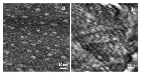
Figure 6.12. Constant-current STM images of Au(111)-films after 30' (a) and 24h (b) of immersion in a freshly prepared THF solution of 5.
