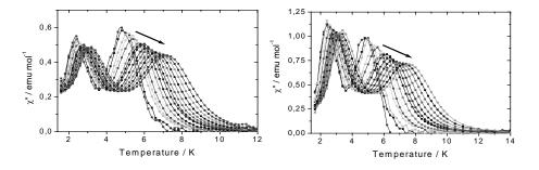
Figure 4.14 Ac out-of-phase signals ( $\chi$ ") at different frequencies (between v=10 and 6580 Hz) for complex 3 (left) and 4 (right).
