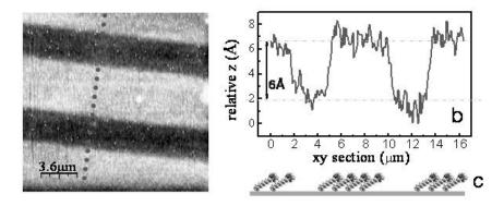
Figure 6.28. (a) AFM image  $(18x18\mu m^2)$  of NIT4 micro-contact printed in stripes on gold with a PDMS stamp (5  $\mu m$  stripes spaced 3  $\mu m$  apart). Dotted line indicates the xy section presented in (b). In (c) a schematic view of the expected packing of molecules on the basis of the measured profiles. Reprinted from Mannini M. et al. 2008b, Copyright 2008, with permission from Elsevier.
