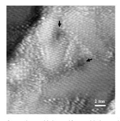
Figure 3.8. STM image of an n-decanethiolate self-assembled monolayer on Au(111) showing two pinhols defects (marked by the black arrows) and multi-domain features.
