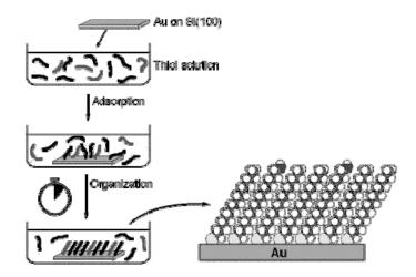
Figure 3.6. Scheme of an n-dodecanethiolate monolayer self-assembling process on an atomically flat gold substrate. Courtesy of P. Tengvall (2000).
