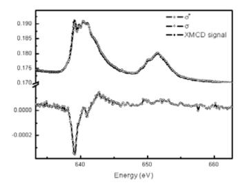
Figure 7.9. XAS spectra and XMCD signal at Mn L<sub>2.3</sub> edges of a monolayer of 2 on gold.
