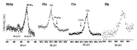
Figure 6.13. XPS core-level spectra for Au(111) films 24h of immersion in THF solution of 5.
