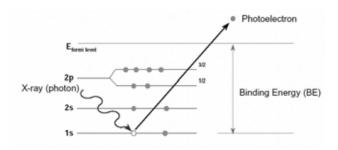
Figure 2.1. Representation of the photoemission process occurring in XPS measurements.
