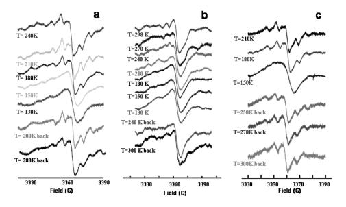
Figure 7.14. Temperature and time evolution of the ESR spectrum of a SAM of NIT1(a), NIT2 (b) and NIT3 (c) deposed on gold. Magnetic field oriented along the normal to the gold slide.
