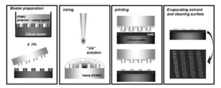
Figure 3.9. µCP technique schematic summary. (From left to right). Stamp preparation from a pre-patterned silicon master. Inking phase. Printing step. Evaporation and cleaning phases.
