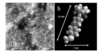
Figure 6.25. In air STM image 50 x 50 nm2 sized of NIT2 SAM on gold surface, a) unfiltered scan,; b) 3D representation of NIT2. Reproduced with permission from Mannini M. et al. 2007b. Copyright 2007 American Chemical Society.
