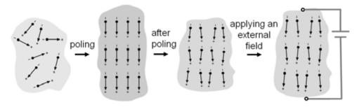
Figure 2.8. Electric dipoles in domains. From left to right: (1) unpoled ferroelectric ceramic, (2) during and (3) after poling piezoelectric ceramic, (4) applying an external electric field. From PI 2005, copyright (2005) Physik Instrumente (PI) GmbH & Co. KG.
