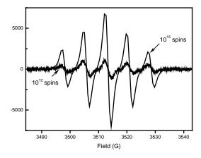
Figure 5.8. Room temperature X-band ESR spectra of NIT3 in  $CH_2Cl_2$  in function of the quantity of spins contained in the examined solutions.
