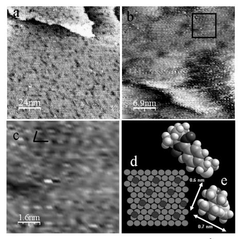
Figure 6.27. In air STM image of NIT3 SAM on gold surface, (a)  $120 \times 120 \text{ nm}^2$  sized unfiltered scan, (b)  $35 \times 35 \text{ nm}^2$  unfiltered scan, (c) digital zoom  $8 \times 8 \text{ nm}^2$  of previous image, the dark lines indicate the suggested primitive cell; (d) the (3x2) suggested packing model; (e) two 3D representations of NIT3. Reproduced with permission from Mannini M. et al. 2007b. Copyright 2007 American Chemical Society.
