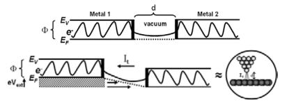
Figure 2.12. Scheme of a two metallic surfaces keep in quasi-contact at the same energy (up) and applying an external potential (down).
