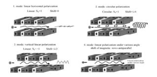
Figure 7.3. Relative arrangement of the magnet arrays achieving differently polarized lights. Courtesy of BESSY, Germany.
