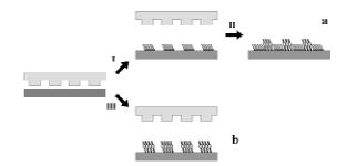
Figure 6.17. Schematic view of the process for indirect (top) and direct (bottom)  $\mu$ CP of SMMs stripes on gold surfaces: I)  $\mu$ CP of thiols, II) deposition of SMMs on a pre-printed surface, III)  $\mu$ CP of SMMs. Reproduced with permission from Mannini M. et al. 2005. Copyright 2005 American Chemical Society.
