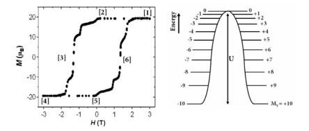
Figure 4.2. (Left) Hysteresis loop recorded at 2.1 K on a single crystal of Mn12-acetate (1), with the magnetic field directed along the tetragonal axis. (Right) Splitting of the S = 10 ground spin state in Mn12-acetate.  $M_S$  is the quantum number. The arrows indicate the successive spin transitions required to overcome the anisotropy barrier U.
