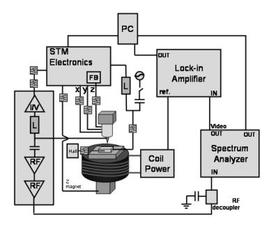
Figure. 8.3. Detection scheme for ESN-STM. The signal (which occurs as a result of a magnetic field) is recovered from the STM tunnelling current and is split into the DC and AC part. The AC part is then amplified and detected by a spectrum analyzer and evidenced through a PSD by the Lock-in Amplifier (if the magnetic field is modulated). Reprinted from Mannini M. et al. 2007a, Copyright 2007, with permission from Elsevier.
