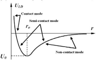
Figure 2.18. Interatomic potential versus distance curve. From Mironov V. L. 2004. Copyright (2004) NT-MDT.
