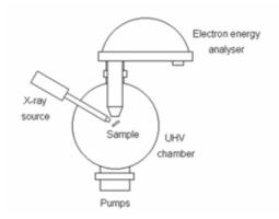
Figure 2.2. Scheme of an XPS apparatus.
