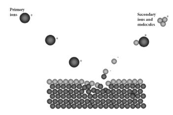
Figure 2.3. Simulation of the impact of primary ion on sample surface and consequent emission of secondary ions.
