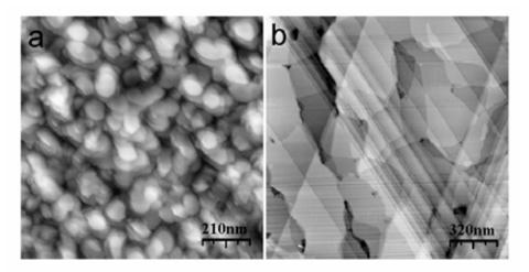
Figure 3.4. STM images of gold deposits evaporated on mica before (a) and after (b) hydrogen flame annealing.
