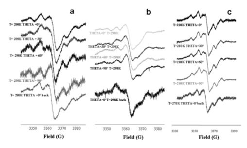
Figure 7.15. Angle dependencies of the ESR spectrum of a SAM of NIT1(a), NIT2 (b) and NIT3 (c) deposed on gold. Theta is the angle within the magnetic field and the normal to the gold slide.
