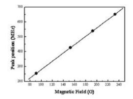
Figure 8.8. Position of ESN-STM peak measured at different values of applied magnetic field. The slope of the best fit line is  $g\mu_B/h$ : the obtained value for g is equal, within experimental error, to 2.0. Reprinted from Mannini M. et al. 2007a, Copyright 2007, with permission from Elsevier.
