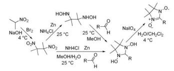
Figure 5.1. Reaction scheme for the synthesis of NIT(R) radicals (Bogani L. 2005). Two possible pathways for the condensation of the aldehyde are represented. See text for details on each step.
