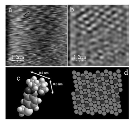
Figure 6.24. In air STM image 5.3 x 5.3 nm<sup>2</sup> sized of NIT1 SAM on gold surface, a) unfiltered scan, the dark lines indicate the primitive cell suggested; b) Filtered with FFT; c) 3D representation of NIT1; d) the (2x2) suggested packing model. Reproduced with permission from Mannini M. et al. 2007b. Copyright 2007 American Chemical Society.
