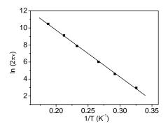
Figure 4.13. Relaxation rate of the magnetization of 2 plotted as a function of inverse blocking temperature.
