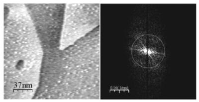
Figure 6.8 (Left) Constant-current STM image of 4 assembled on the Au(111) surface (scan area  $180 \times 180 \text{ nm}^2$ ) showing terraces and a triangular features typical of Au(111) reconstruction on mica. (Right) 2D-FFT of the image on left. Hexagonal regularity with features between 6 and 8 nm.
