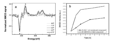
Figure 7.12. (a) XMCD signal at Mn  $L_{2,3}$  edges of a monolayer of 4 on gold deposed from dichloromethane varying the external magnetic field. (b) Dependences with the magnetic field of the most significative peaks (marked with asterisks) observed in (a).
