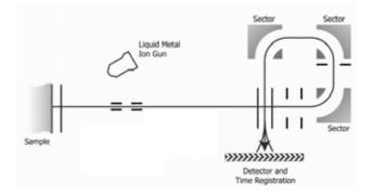
Figure 2.5. TRIFT III (ToF) spectrometer simplified scheme.
