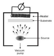
Figure 3.1. Scheme of a metal evaporator.
