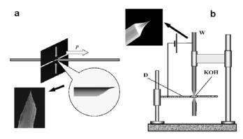
Figure 2.14. Preparation of the tips using mechanical cutting (a) and electrochemical etching (b). From Mironov V. L. 2004, copyright (2004) NT-MDT. On the inset are presented SEM images of prepared tips.
