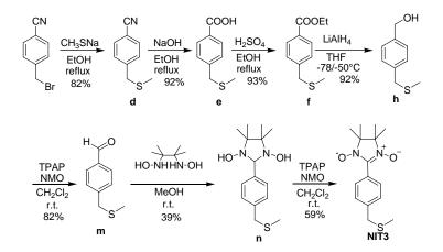
Figure 5.6. Scheme of the preparation of NIT3.
