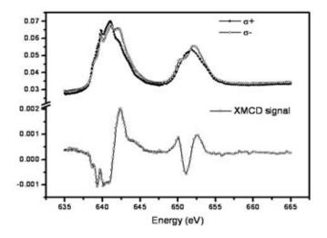
Figure 7.6 XAS spectra and XMCD signal at Mn L<sub>2.3</sub> edges in bulk 4.
