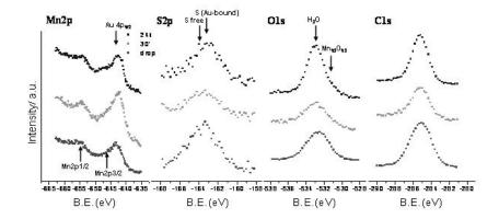
Figure 6.2. XPS core-level spectra of Au(111) films after 30' (middle, light gray) and 24h (down, dark gray) of immersion in a 24hrs old THF/NH<sub>3</sub>(aq) solution of 2, compared to a a bulk deposition obtained by drop-casting using a saturated solution of 2 in  $CH_2Cl_2$  (up, black). The spectra of each element are on the same absolute scale.
