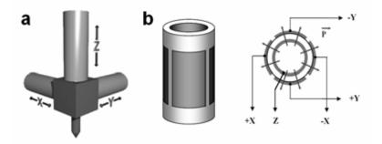
Figure 2.9. (a) Tripod Scanner scheme. (b) Tube scanner scheme and electrodes connections. From Mironov V. L. 2004. Copyright (2004) NT-MDT.
