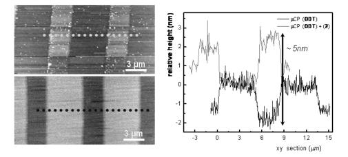
Figure 6.18. AFM images  $(20x10\mu m^2)$  of ODT micro-contact printed in stripes on gold (down-left) and of the alternating pattern of ODT and 2 (up-left). Dotted lines indicate the sections in the xy plane presented on the right. The height of 2 has been obtained by setting the top of the ODT stripes at zero height. Reproduced with permission from Mannini M. et al. 2005. Copyright 2005 American Chemical Society.
