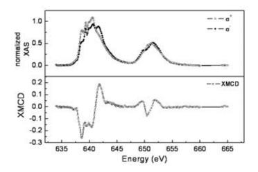
Figure. 7.7. XAS spectra and XMCD signal at Mn L<sub>2,3</sub> edges of drop cast 4 on gold.
