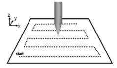
Figure 2.10. Raster movement scheme of displacement of the tip in respect of the sample.
