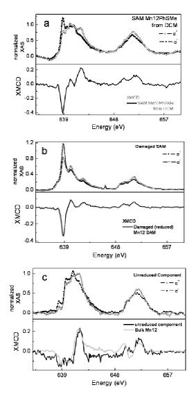
Figure 7.11. (a) Untreated XAS spectra and XMCD signal at Mn  $L_{2,3}$  edges of a monolayer of 4 on gold deposed from dichloromethane. (b) Untreated XAS spectra and XMCD signal at Mn  $L_{2,3}$  edges of a monolayer of the damaged sample which preparation is described in (Fleury B. et al. 2005). (c) Elaborated XAS spectra and XMCD signal at Mn  $L_{2,3}$  edges of a monolayer of 4 on gold after the removal of the supposed MnII contribution derived from (b).
