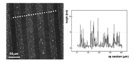
Figure 6.19. (Left) AFM image (50x50 m<sup>2</sup>) of 2 micro-contact printed in stripes on gold with a PDMS stamp (5  $\mu$ m stripes spaced 3  $\mu$ m apart). Dotted line indicates the xy section pre-
