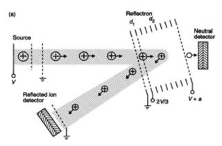
Figure 2.4. A simplified scheme of a ToF detector.
