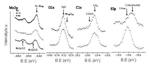
Figure 6.10. XPS core-level spectra for Au(111) films after 30' (middle, light gray, only for Mn2p) and 24h (up, dark gray) of immersion in THF solution of 4, and of a bulk deposition obtained by drop-casting (down, black) using a saturated solution of 4 in  $CH_2Cl_2$ . The spectra of each element are on the same absolute scale.
