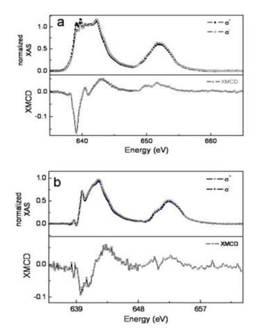
Figure. 7.10. (a) Untreated XAS spectra and XMCD signal at Mn  $L_{2,3}$  edges of a monolayer of 4 on gold. (b) Elaborated XAS spectra and XMCD signal at Mn  $L_{2,3}$  edges of a monolayer of 4 on gold after the removal of MnII contribution.
