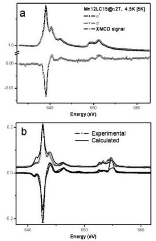
Figure 7.8. (a) XAS spectra and XMCD signal at Mn L2,3 edges of a monolayer of 2 on gold deposited after the treatment of the solution with ammonia. (b) Simulated and recorded spectra obtained for a MnII based compound in an octahedral geometry. Experimental data are obtained from the investigation of  $[Mn(Me_6[14]ane-N_4)Cu(oxpn)](CF_3SO_3)_2$ .
