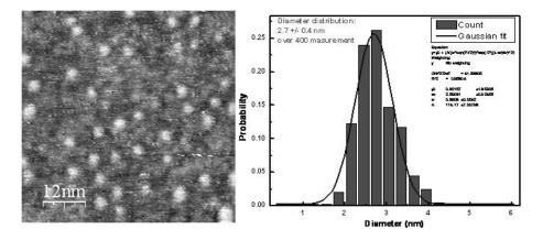
Figure 6.7. (Left) Constant-current STM image of 4 assembled on the Au(111) surface (scan area 60 x 60 nm<sup>2</sup>) after 30' of immersion in a freshly prepared THF solution of 4. (Right) The distribution of diameters extracted from 400 measurements. The best-fit gaussian distribution is shown ( $R^2 = 0.97$ ,  $x_c = 2.7$  nm,  $\sigma = 0.5$  nm). Reproduced with permission from Zobbi L. et al 2005. Copyright 2005 of the Royal Society of Chemistry.
