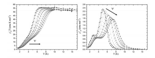
Figure 4.19 Plot of the in-phase, as  $\chi'_{M}$  T, and out-of-phase,  $\chi''_{M}$ , ac susceptibility signals vs. temperature for complex 6 at different oscillation frequencies between 100 and 6580Hz.
