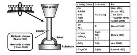
Figure 3.5. Typical scheme of molecules for SAMs.
