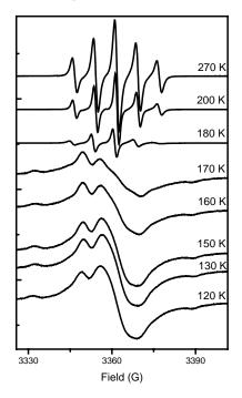
Figure 5.7. X-band ESR spectra of NitPhCH<sub>2</sub>SMe in  $CH_2Cl_2$  in function of the temperature of the solution.
