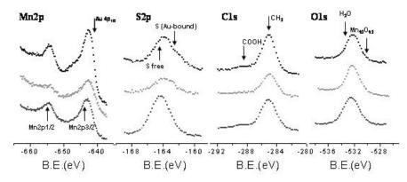
Figure 6.6. XPS core-level spectra for Au(111) films after 30' (middle, light gray) and 24h (up, dark gray) of immersion in a freshly prepared THF/NH<sub>3</sub>(aq) solution of 3, and of a bulk deposition (down, black) obtained by drop-casting using a saturated solution of 3 in  $CH_2Cl_2$ . The spectra of each element are on the same absolute scale.
