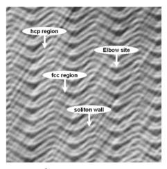
Figure 6.9. STM image (50 x 50  $\text{nm}^2$ ) of "herringbone" reconstructed Au(111) surface showing periodically arranged stress domains separated by soliton walls and a secondary structure of the solitons (herringbone) with partial dislocations (elbow sites).
