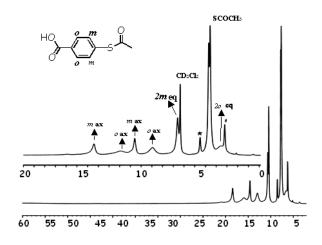
Figure 4.7.  $^{1}$ H-NMR spectrum of a CD<sub>2</sub>Cl<sub>2</sub> solution of 3. The asterisks are used to mark residual Et<sub>2</sub>O .
