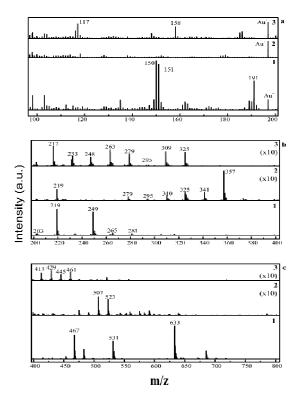
Figure 6.22. Positive ToF-SIMS spectra of SAMs of NIT1, NIT2, and NIT3 on gold. The mass regions between (a) 100 m/z and 200 m/z, (b) 200 m/z and 400 m/z (c) 400 m/z and 800 m/z are presented. In (a) and in (b) the intensity of the NIT2 and NIT3 spectra is amplified 10 times. Reproduced with permission from Mannini M. et al. 2007b. Copyright 2007 American Chemical Society.
