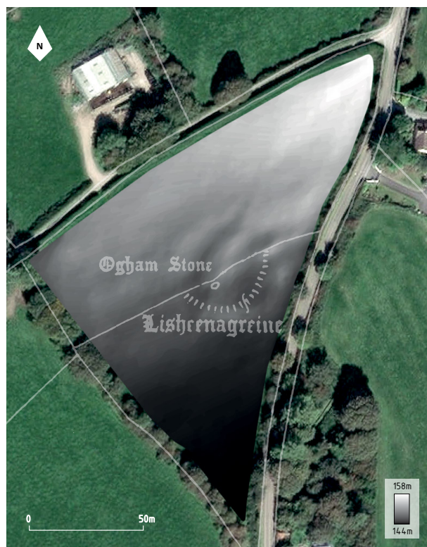
Figure 2.22 Surface model derived from GNSS survey data shows the low-relief remains of Lisheenagreine ringfort. Detail adapted from the Ordnance Survey 1943 map edition is overlain and depicts the reported location of the ogham stone find and the former line of an early modern field boundary running across the monument. (background image: Google, Maxar Technologies)
