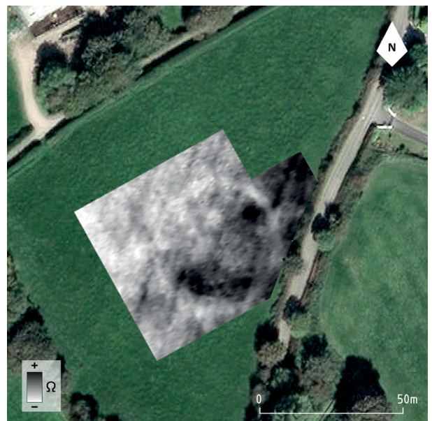
Figure 2.24 Results of electrical resistance survey at Lisheenagreine ringfort. (background image: Google, Maxar Technologies)
