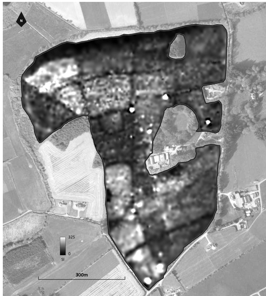
Figure 2.26 Interpolated surface showing results of the magnetic susceptibility survey. (background image: Google, Maxar Technologies)
