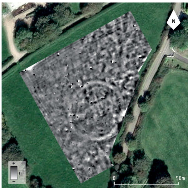
Figure 2.23 Results of magnetic gradiometer survey at Lisheenagreine ringfort. (background image: Google, Maxar Technologies)
