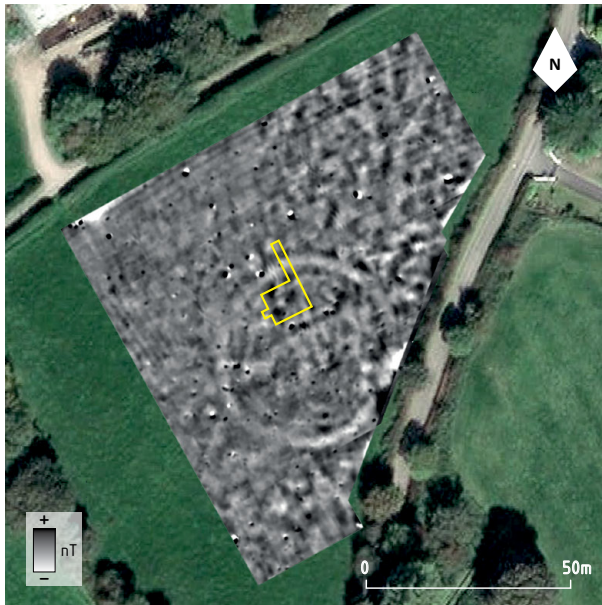
Figure 5.4 Results of magnetic gradiometry survey at Lisheenagreine with location of excavation trenches.
