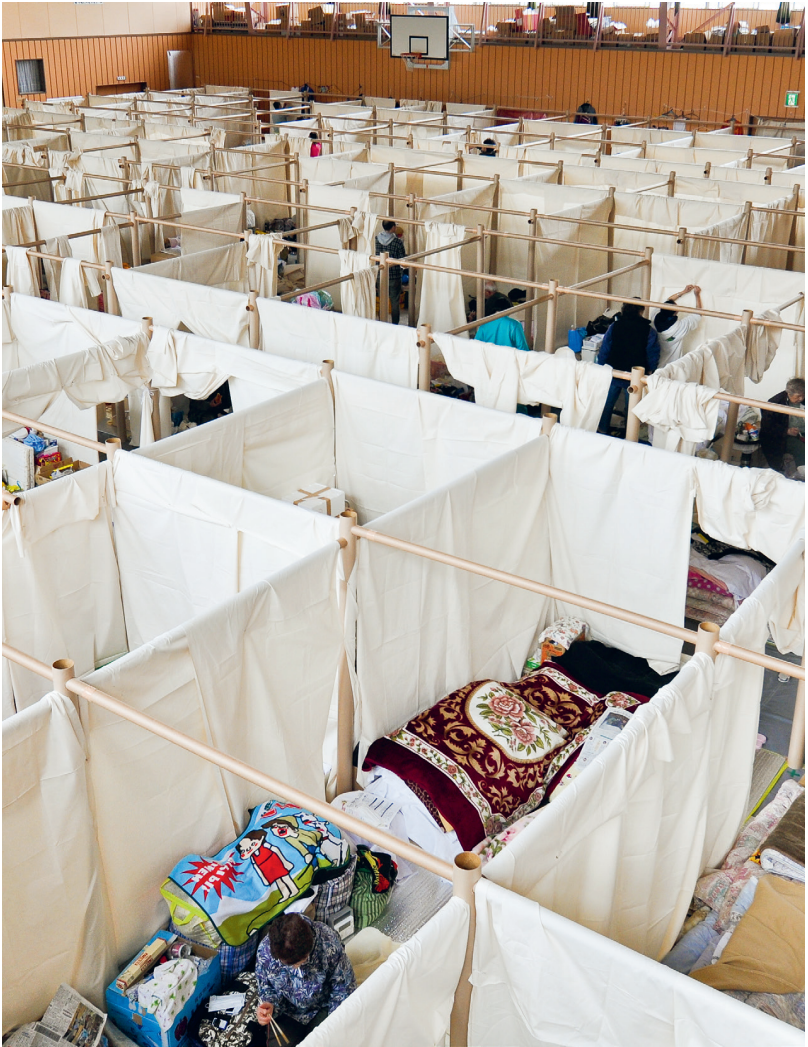
Paper Partition System 4, developed by Shigeru Ban in response to the 2011 earthquake in Japan, is a modular wall system using cardboard tubes and fabric providing privacy in emergency shelters.
