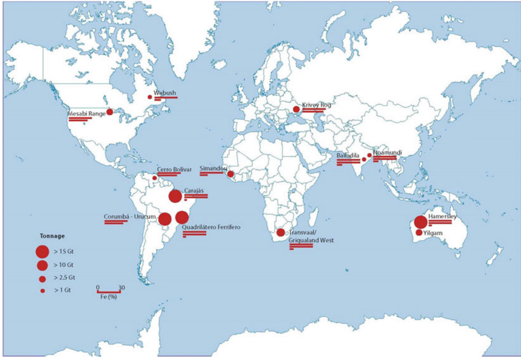
Fig. 1 Location of significant BIF-hosted iron ore districts and deposits. The cumulative length of the bar graphs beneath each locality indicates the Fe grade
