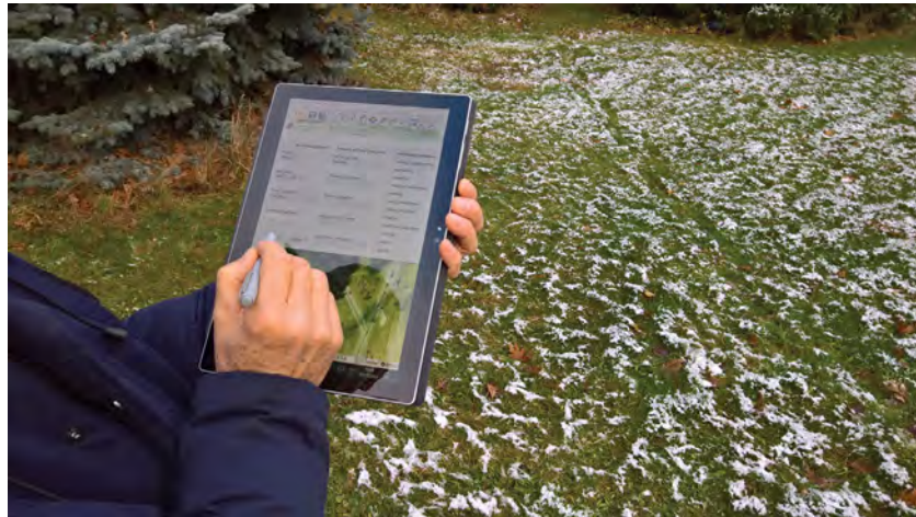
Figure 6.9 A photo showing how the GIS digital interface is operated on a tablet computer on site. Here the drop-down menu for recording the attributes of someone using the site is open over the map base (Source: Peeter Vassiljev)
