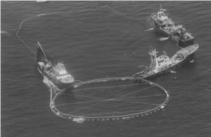
Fig. 10.4. A Spanish trawler hauling in a purse seine full of small tuna that will be transferred to the cage in the foreground and then towed to a tuna pen in Malta for fattening (photo: Steven Vella).
