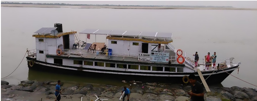
Figure 14.3 The boat clinics within which all health and general appliances are energy-efficient and solar powered.
