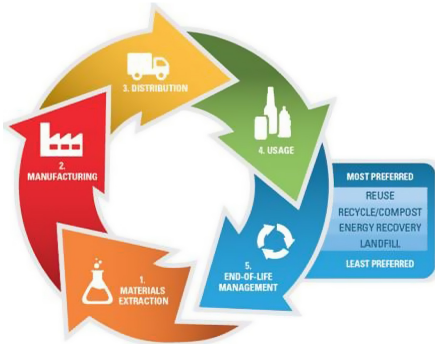
Figure 18.1 Lifecycle of materials and products from material extraction, manufacturing, distribution and use till end-of-life.
