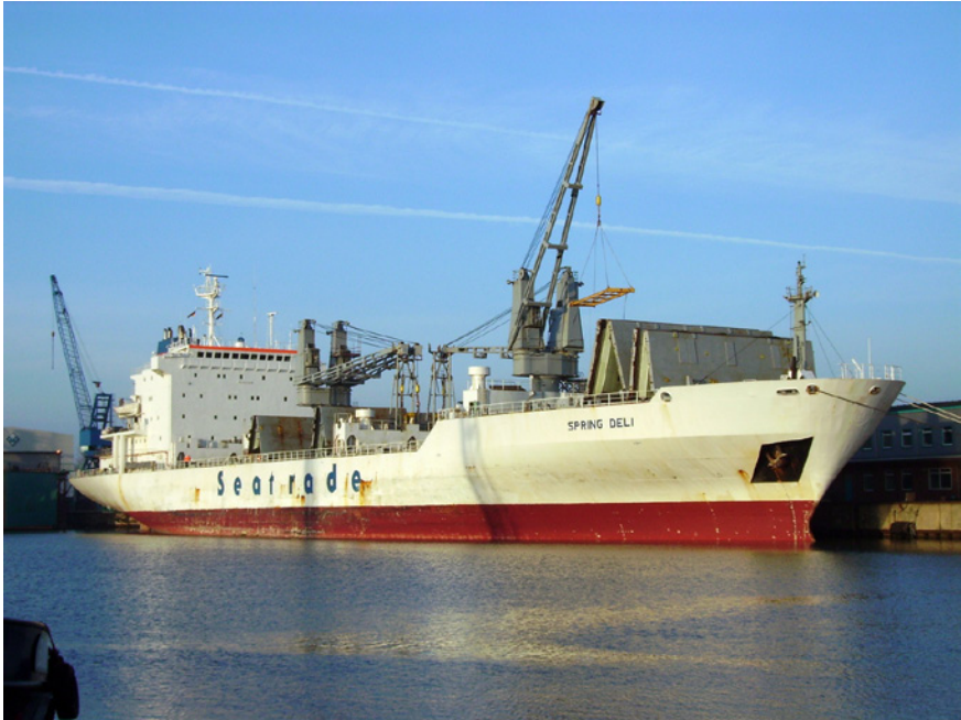
FIGURE 7 Spring Deli, previously Spring Delight, later sailed for Seatrade. Note the massive hatches folded up ondeck
