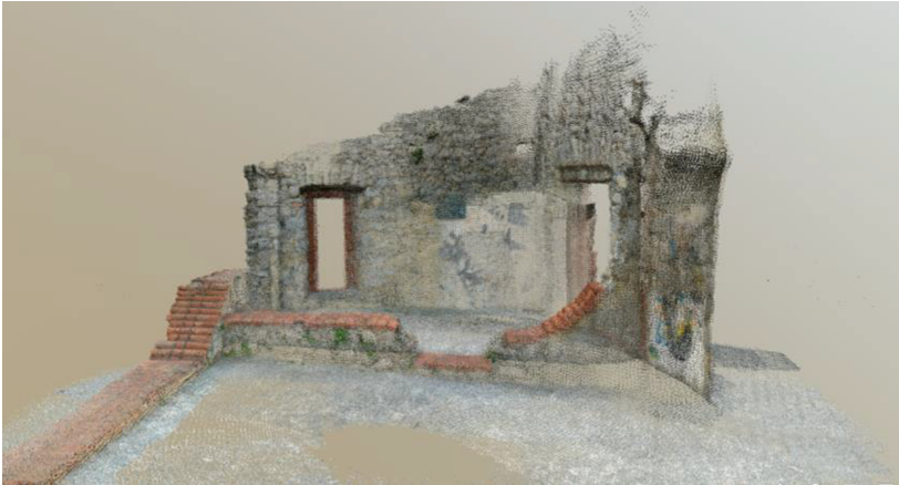
Fig. 3. 3D model reconstructed using RTAB-Map [18]
