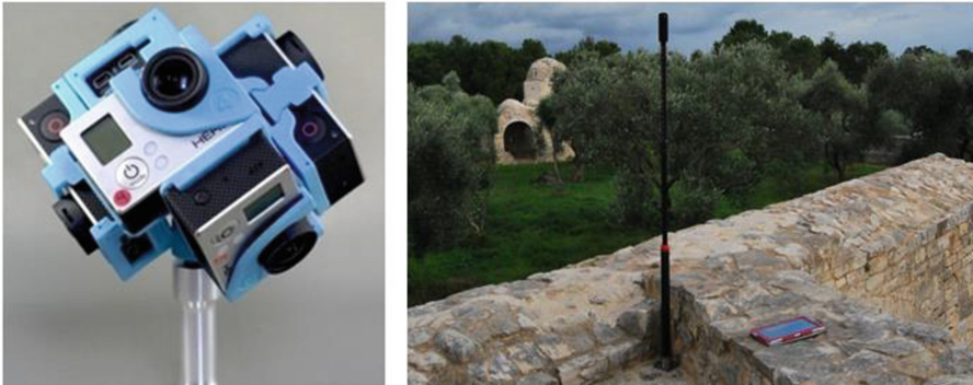
Fig. 3. 360-degree systems: Commercial six camera spherical array specifically designed (left—source: Aerial Technology International, Oregon City, United States); Ricoh Teta Plus mounted on a telescopic rod in carbon fiber, with a cylindrical, low-radius, heavy base specifically designed to reduce its footprint (right).
