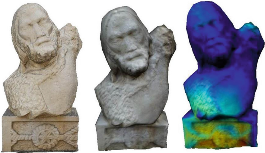
Fig. 11. Photogrammetry reconstructed 3D model (a) Tango reconstructed 3D (b) Photogrammetry/Tango models Hausdorff distance computed for the Tango based model (c)
