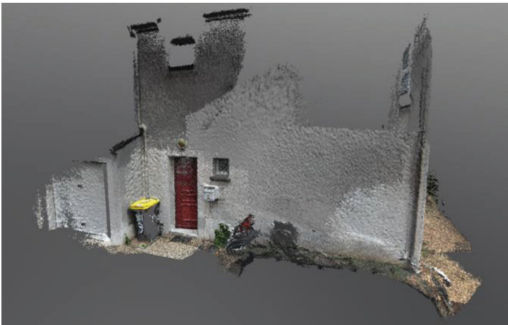
Fig. 4. 3D model reconstructed using Matterport Scenes [25]
