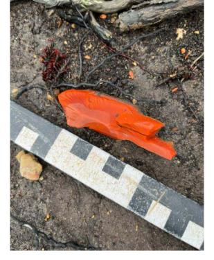
Unburnt propellant in and around the wreckage (credit: Falklands War Mapping Project)
