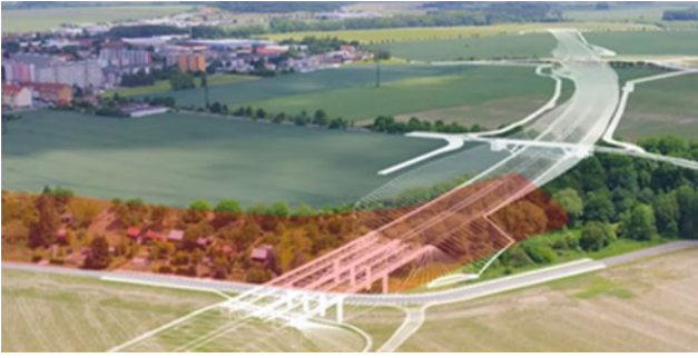
Fig. A.21 Landslide (in red) in the way of the planned motorway D35 in eastern Czechia
