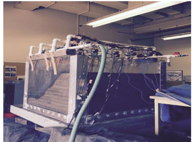
Fig. 7 Custom designed sprinkler system used for this study
