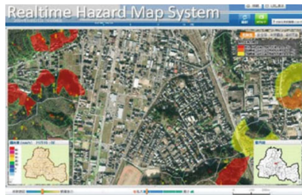
Fig. A.41 Our realtime hazard map reflects up-to-date information of soil natures and precipitations at landslide hazard sites, etc. that can constantly be changing, and evaluates area-wide hazard risk in real-time
