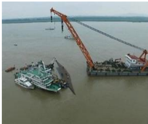
The righting of the capsized cruise ship
