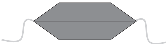
Figure 2.2 Gull-wing leaded plastic package (not to scale).
