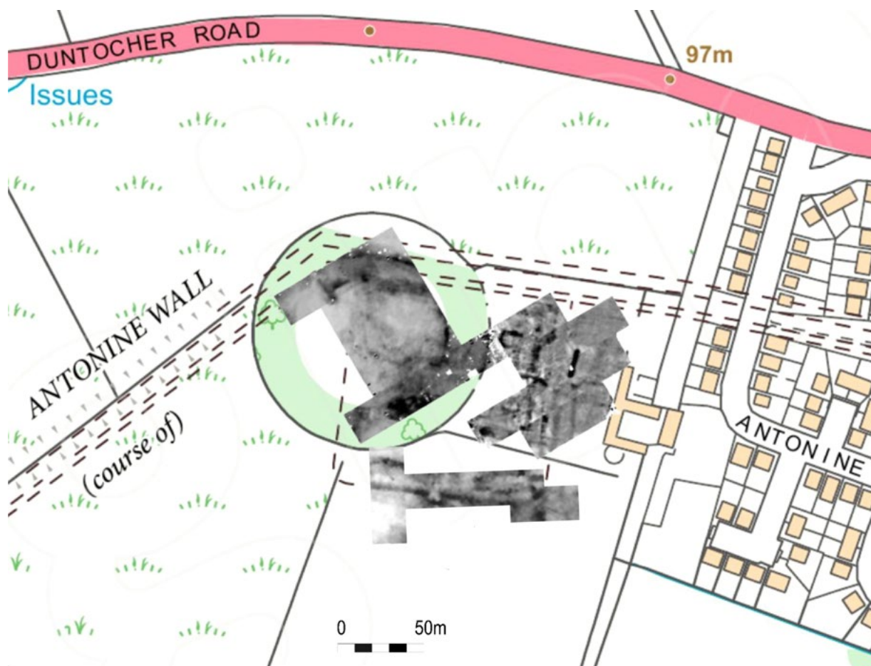
Figure 15.3. Location plan of the resistivity surveys. The main survey to the north was undertaken in 2008; the coverage of the southern defences was obtained in 2019
